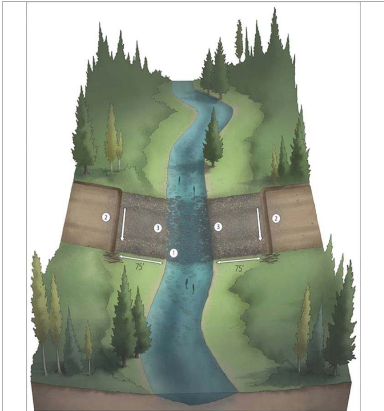
Rocked ford should be oriented perpendicular to the watercourse (1). Rolling dips installed 75' from watercourse (2). Angular rip-rap used to construct ford with angular gravel used for the approaches. (Image: Kroese)
