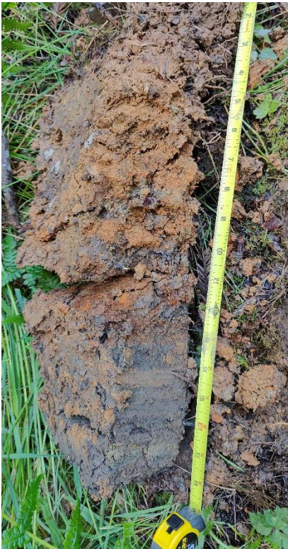
Photo 2. Hydric soil profile with gray, depleted matrix underlying reddish orange soil surface layer (probably fill used to level site).
