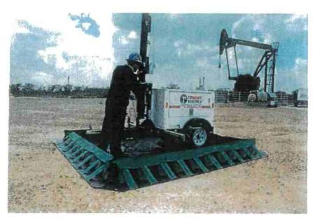
Example of a small, portable, and compact containment berm.
