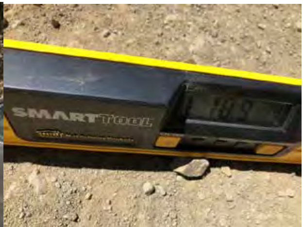
Photo #183 Red Rock Rd Looking Northwest @ Curve w/ Pullout Photo #184 Red Rock Rd Slope is 18.9%
