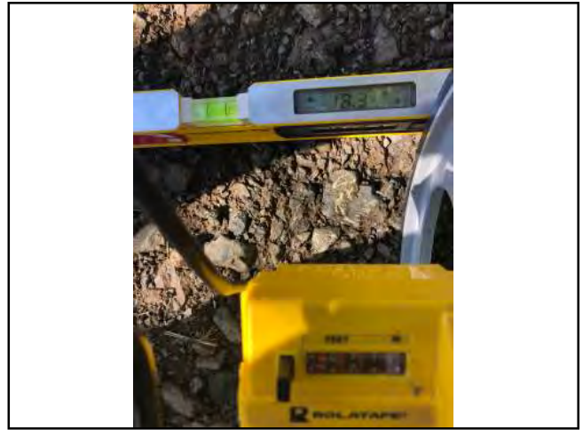
Photo #50 Road H Slope 18.3% Width 11'7"
