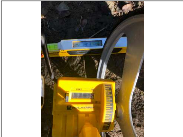
Photo #27 Fish Canyon Rd Slope 13.% Width 13'2"
