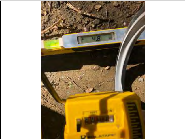
Photo #93 Road H Slope 4.8% Width 11'0"
