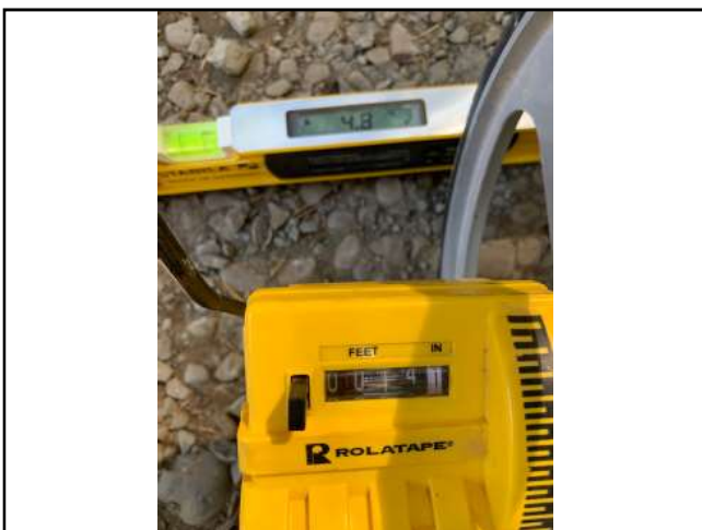
Photo #65 Private Access Rd Slope 4.8% Width 14'1"
