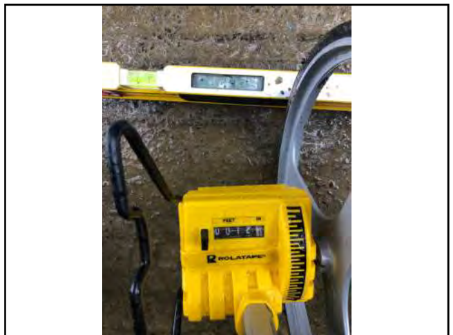
Photo #6 Unnamed Rd Slope 7.4% Width 12'1"
