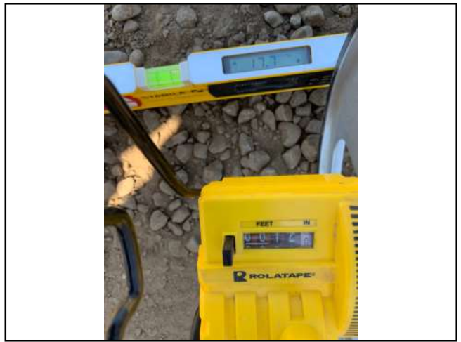
Photo #56 Private Access Rd Slope 17.7% Width 12'8"
