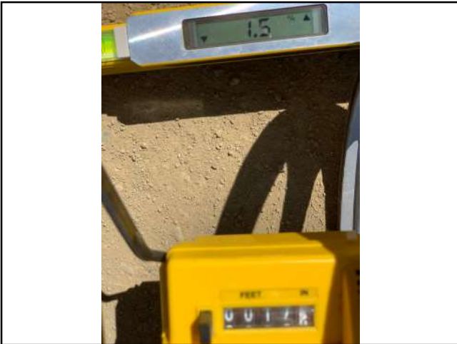
Photo #105 Unnamed Rd Slope 1.5% Width 17'8"
