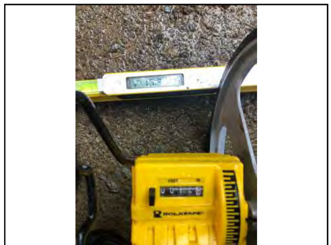
Photo #24 Unnamed Rd Slope 17.3% Width 12'3"
