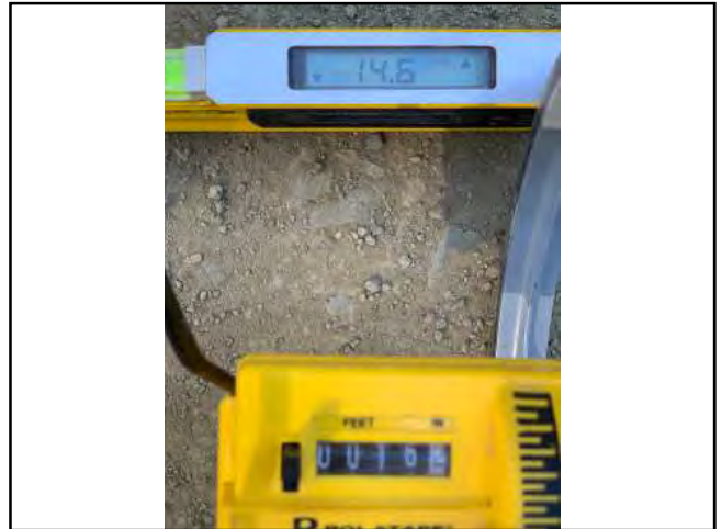
Photo #100 Unnamed Rd Slope 14.6% Width 16'2"
