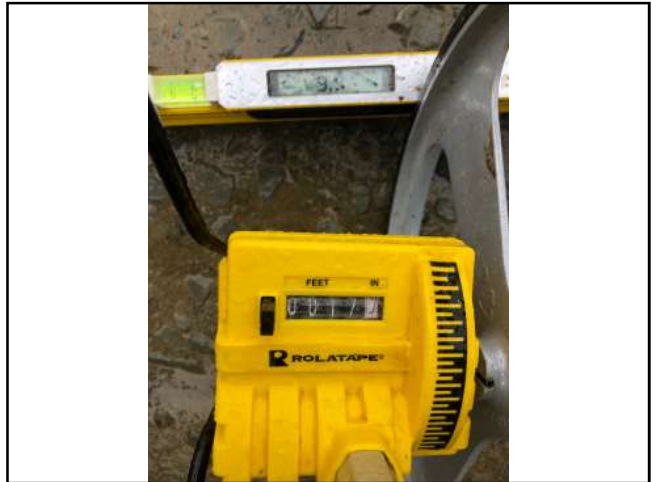
Photo #10 Unnamed Rd Slope 9.9% Width 17'7"
