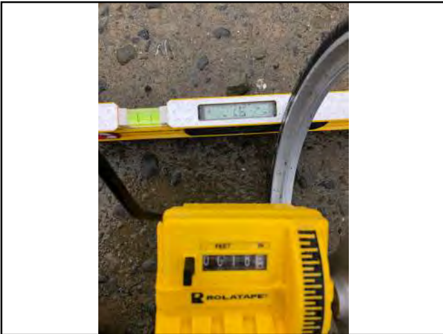
Photo #3 Unnamed Rd Slope 1.6% Width 18'3"
