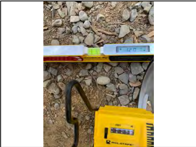
Photo #69 Private Access Rd Slope 12.0% Width 12'8"
