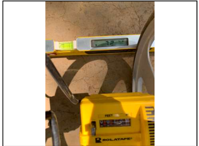
Photo #88 Private Access Rd Slope 7.2% Width 13'1"
