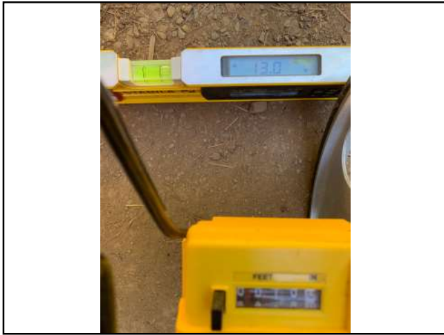
Photo #73 Private Access Rd Slope 13.0% Width 13'6"
