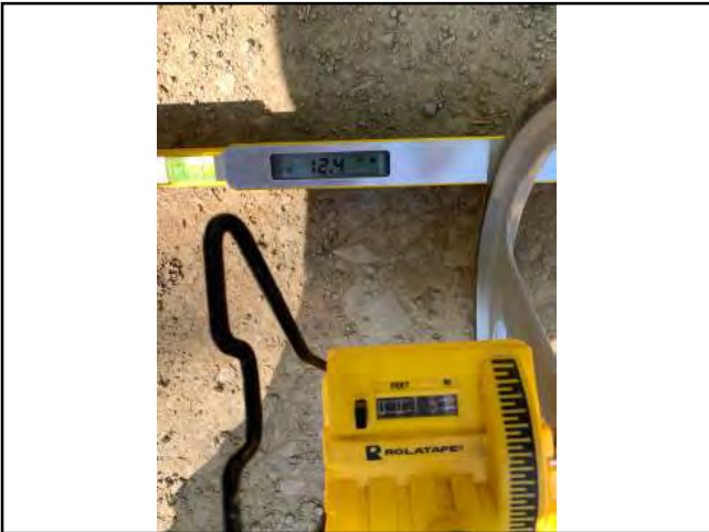
Photo #135 Unnamed Rd Slope 12.4% Width 15'11"
