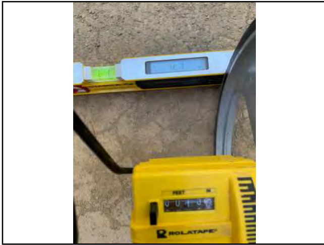
Photo #91 Unnamed Rd Slope 4.7% Width 13'5"
