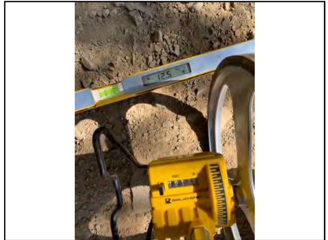
Photo #94 Unnamed Rd Slope 12.5% Width 13'7"
