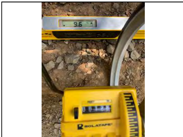
Photo #77 Private Access Rd Slope 9.6% Width 12'2"
