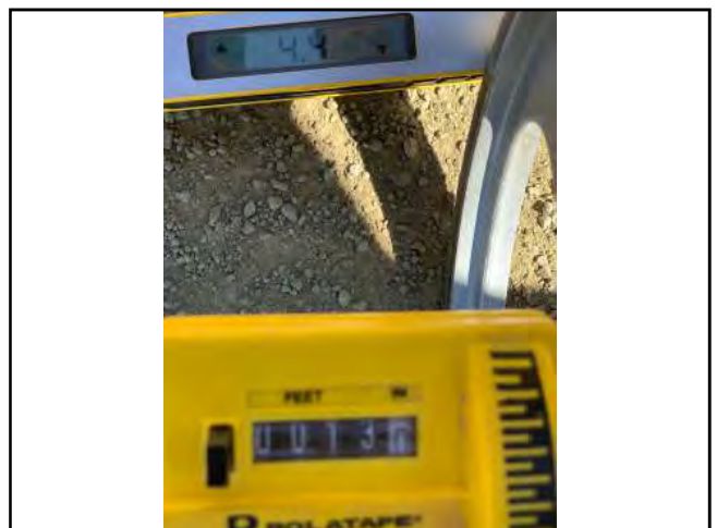
Photo #108 Unnamed Rd Slope 4.4% Width 13'0"
