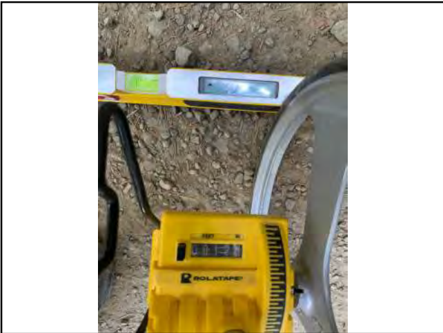
Photo #141 Unnamed Rd Slope 5.3% Width 12'3"
