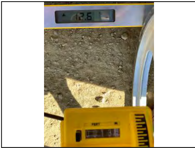
Photo #121 Unnamed Rd Slope 12.6% Width 13'6"
