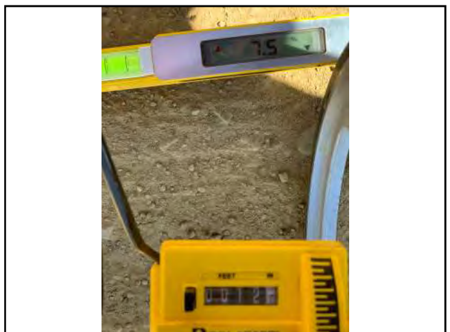
Photo #114 Unnamed Rd Slope 7.5% Width 12'10"
