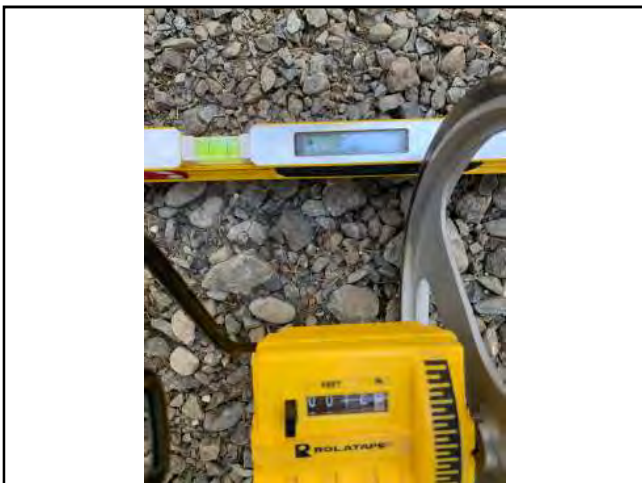
Photo #83 Private Access Rd Slope 6.3% Width 12'1"
