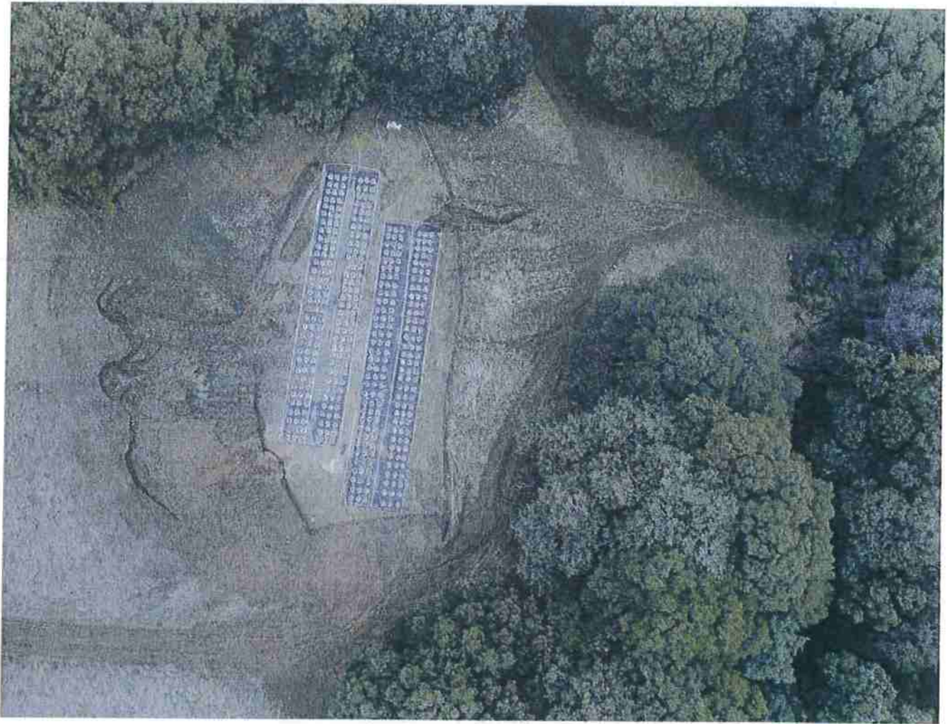
Picture 2: Cultivation site proposed for relocation. Note cut-slope failures above the site, and fill-slope erosion and debris torrent below the site. Photo date 3-1-2019.
