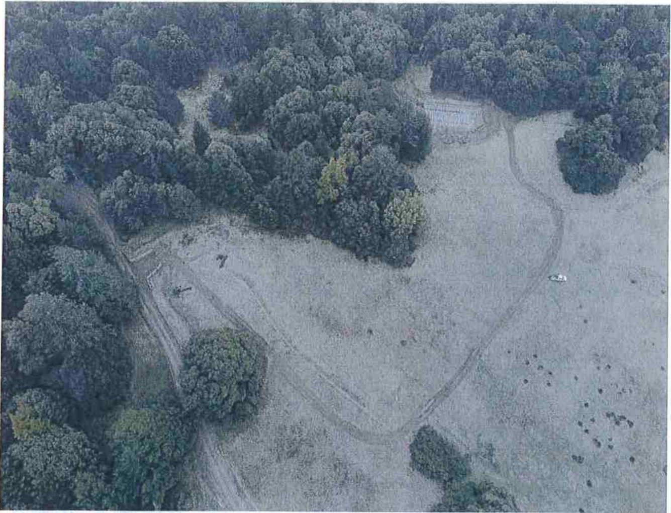
Picture 4: Seasonal road accessing the cultivation site proposed for relocation and restoration. The access road shall be abandoned via the installation of waterbars to a spacing consistent with a "high" Erosion Hazard Rating per 14CCR 914.6. Photo date 3-1-2019.
