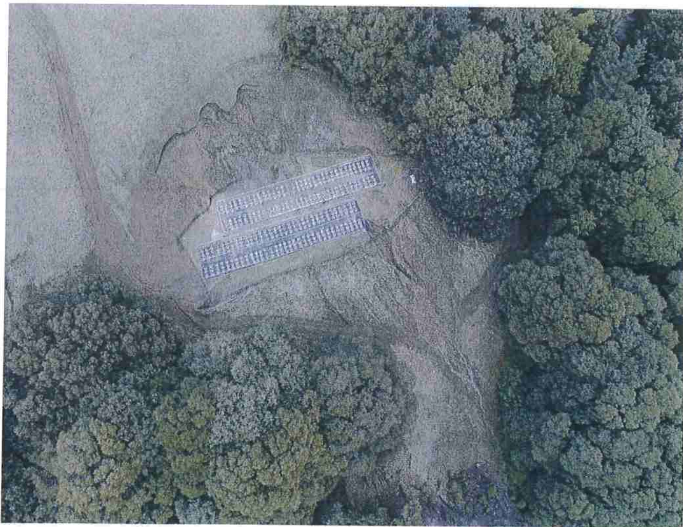
Picture 1: Cultivation site proposed for relocation. Note cut-slope failures above the site, and fill-slope erosion and debris torrent below the site. Photo date 3-1-2019.
