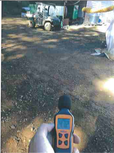
Photo taken at observation point OB50ft showing that the decibel reading is at 47.2 dBA.
