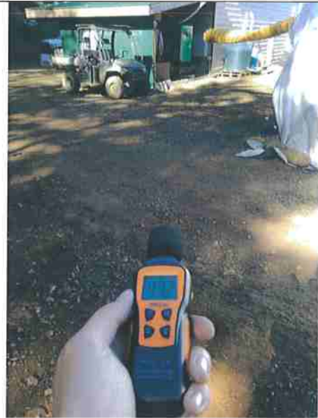
Additional photo taken at observation point OB50ft showing that the decibel reading is at 47.2 dBA.
