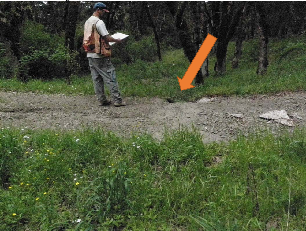
Photo 4- Downstream view of Stream Crossing (SC) #1- looking at the road bed. SC#1 is a fill crossing on Class III watercourse with no formal drainage structure. Note the small headcut at the outboard road (Photo April 2016).
