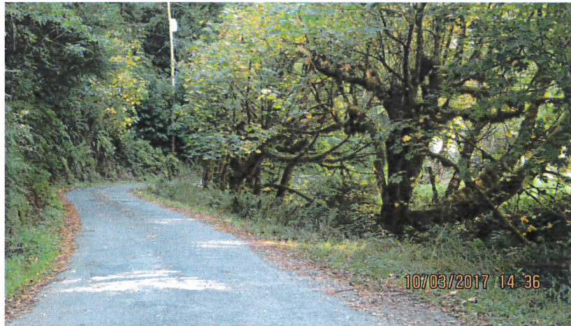
Photo 1662. Milepost 0.69. Single-lane section. Inadequate sight distance on S-curve owing to maple trees along Essex Gulch Creek.
