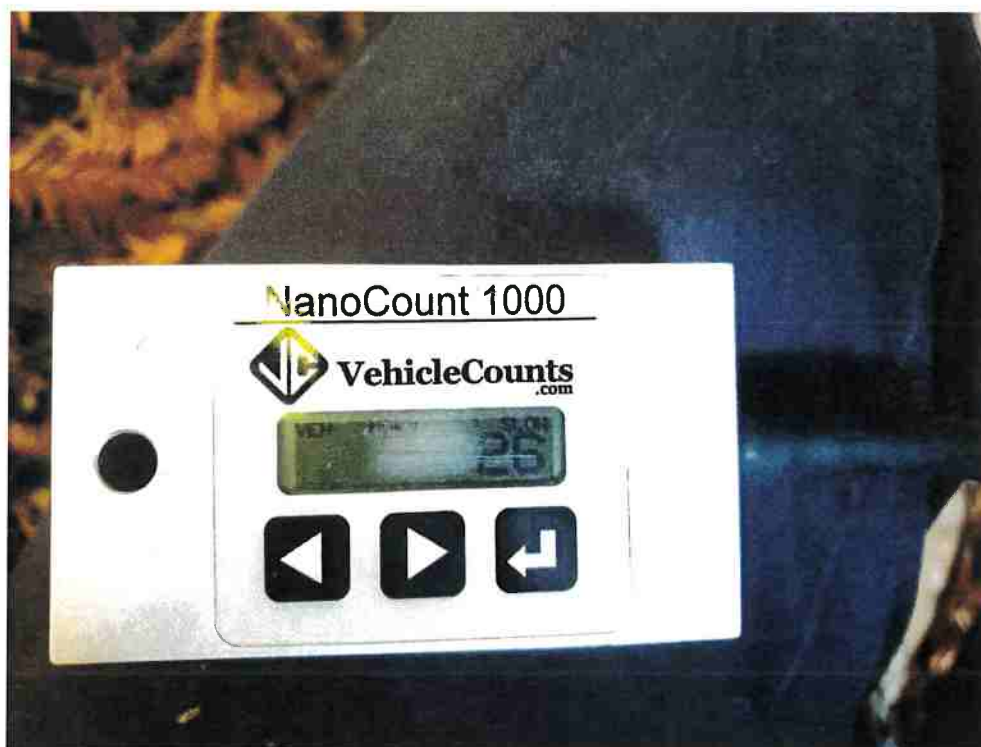
Figure 25: Nanocount 1000 used for 24-hour road study on Warren Creek Road at <124°1'30.689"W 40°53'37.41"N> from 11/20/2019 to 11/21/2019, showing final reading of 26 vehicles
