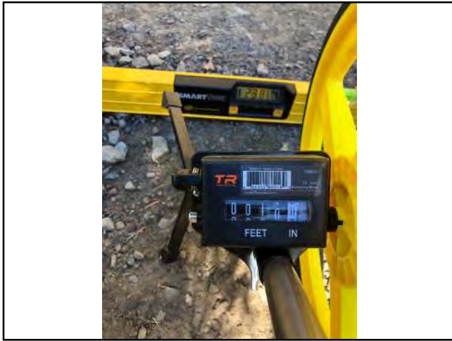
Photo #324 Private Access Rd APN 208-231-004 Slope 23.8% Width 10'11"
