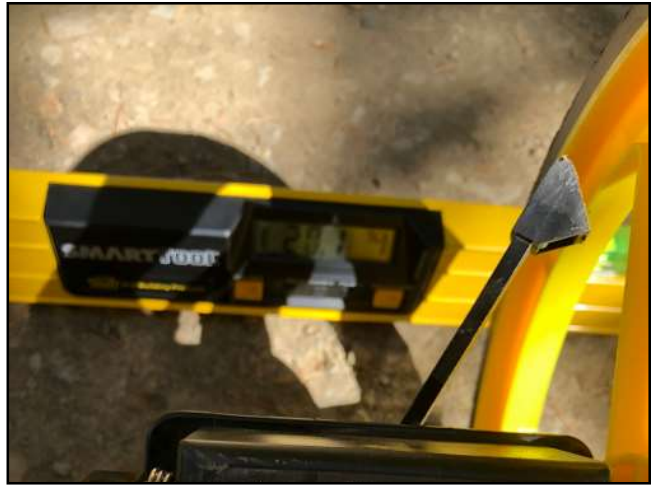
Photo #343 Private Access Rd APN 208-231-004 Slope 20.1 Width 12'2"
