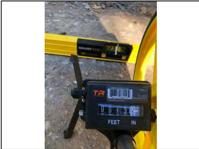
Photo #326 Private Access Rd APN 208-231-004 Slope 27.2% Width 13' 2"
