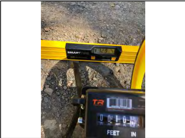
Photo #302 Private Access Rd APN 208-231-004 Slope 12.9% Width 10'0"
