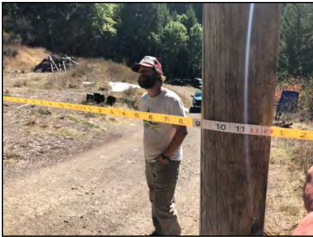
Photo #306 Private Access Rd APN 208-231-004 @ Gate Location Width 10'9"
