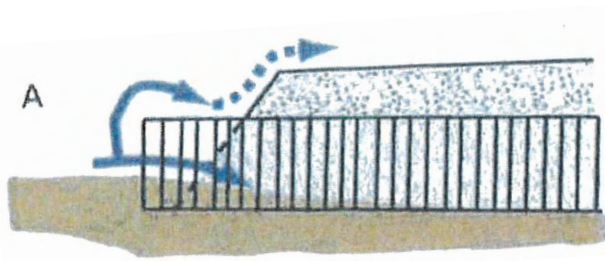
FIGURE 155. Proper culvert installation involves correct culvert orientation, setting the pipe slightly below the bed of the original stream, and backfilling and compacting the fill as it is placed over the culvert. Installing the inlet too low in the stream (A) can lead to culvert plugging, yet if set too high (B) flow can undercut the inlet. If the culvert is placed too high in the fill (C), flow at the outfall will erode the fill. Placed correctly (D), the culvert is set slightly below the original stream grade and protected with armor at the inlet and outlet. Culverts installed in fish-bearing stream channels must be inset into the streambed sufficiently (>25% embedded) to have a natural gravel bottom throughout the culvert (Modified from: MDSL, 1991).
