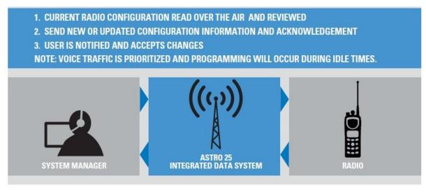
Figure 5-6: Over-the-Air Programming Steps
