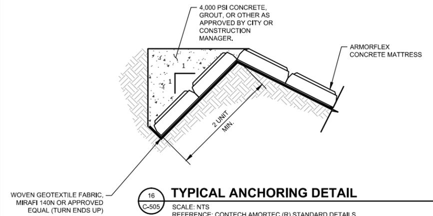
16 TYPICAL ANCHORING DETAIL
