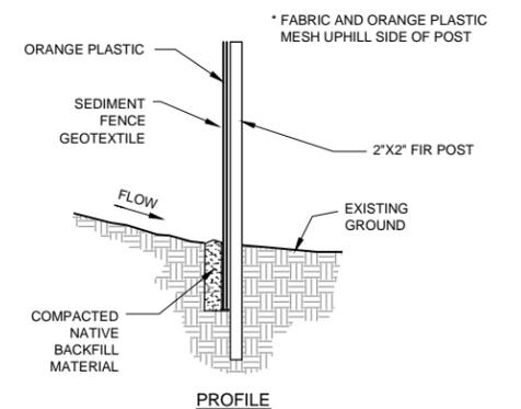
4. TRENCH SHALL BE BACKFILLED WITH NATIVE MATERIAL.
