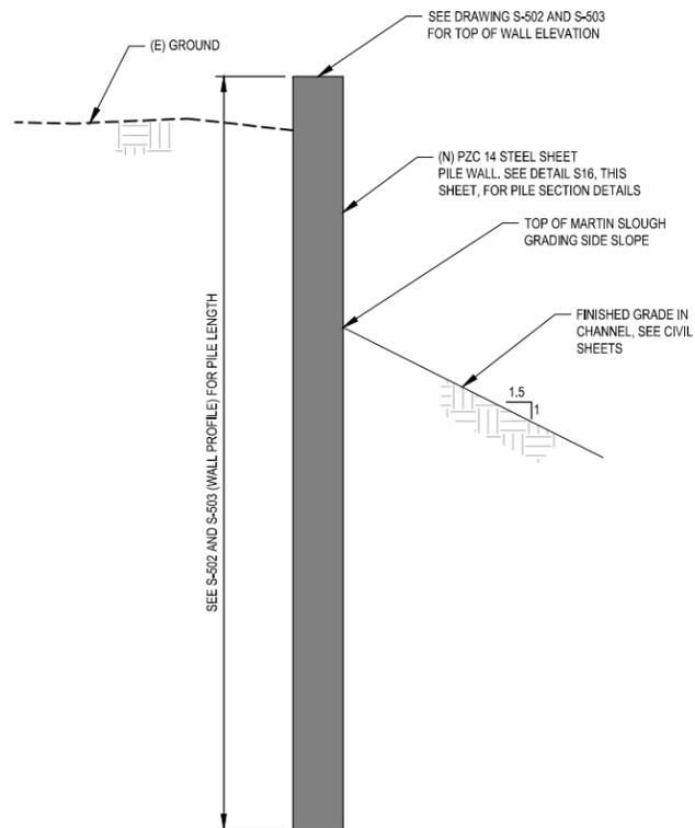
**S15** SHEET PILE SECTION DETAIL
