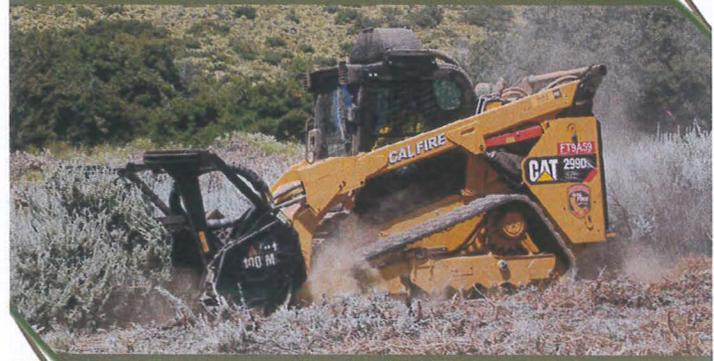
Using the skid steer with attachments, an operator can cut and masticate small and medium sized trees, remove and pile brush, and move piles of cut material to a central location for pile burning or removal.
