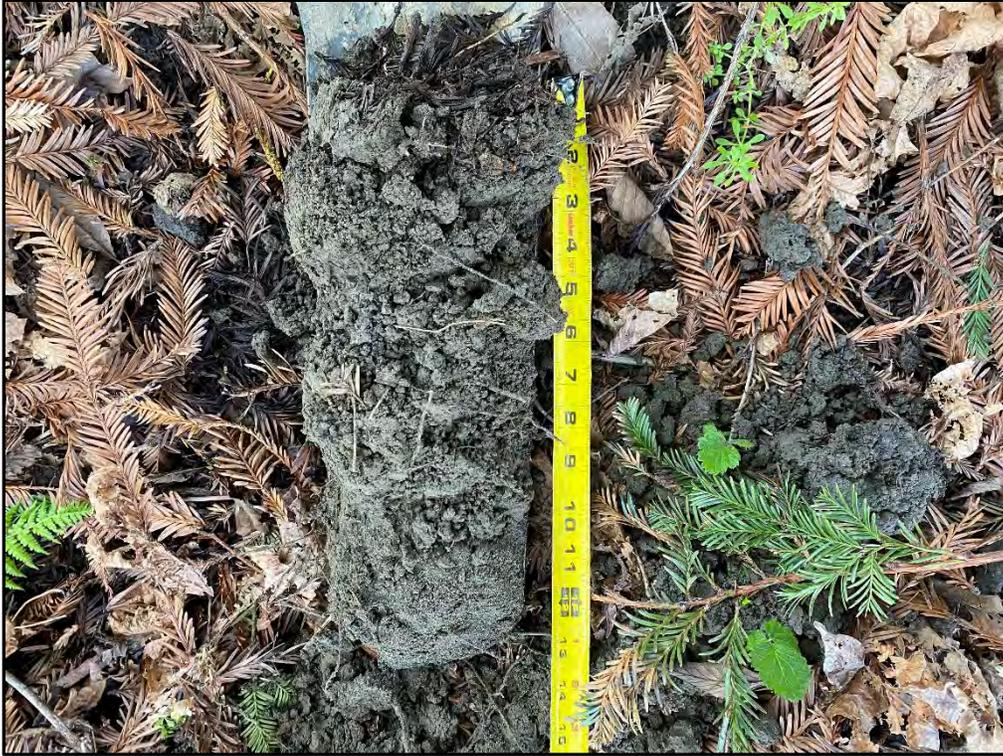
**Photo 11.** View of the soil profile at TP-6 lacking hydric soil indicators.
