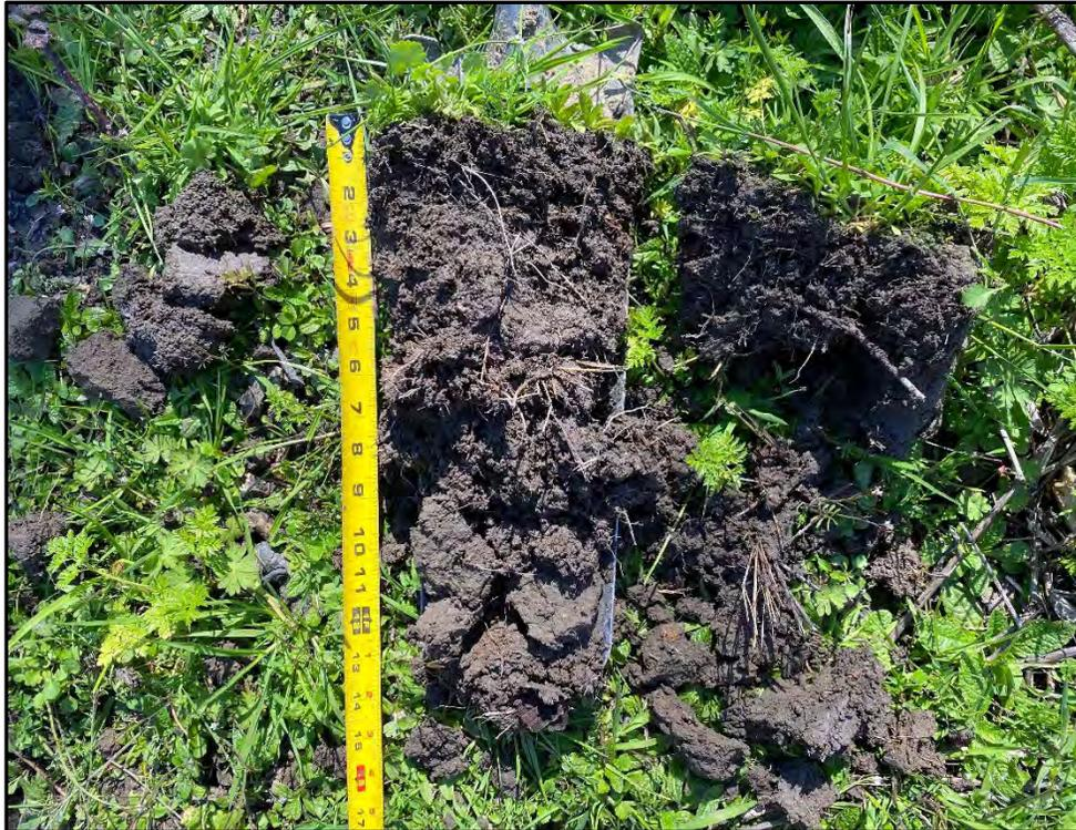
**Photo 13.** View of the soil profile at TP-7 lacking hydric soil indicators.
