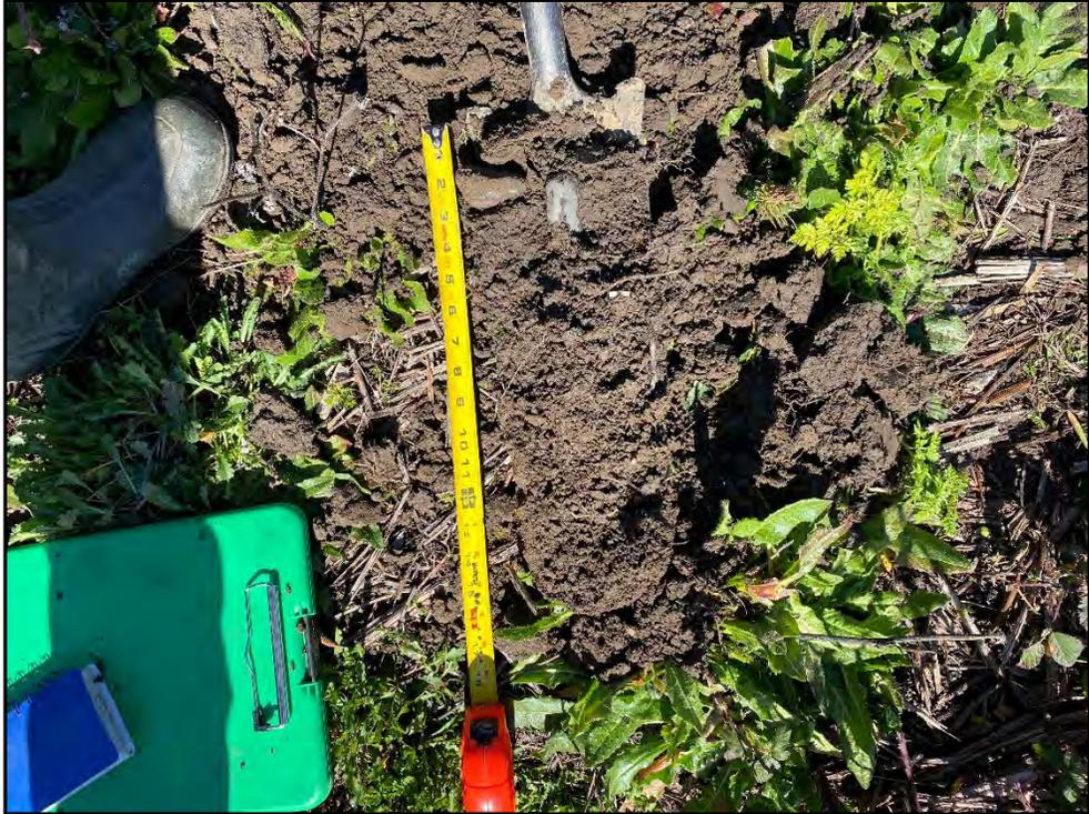
**Photo 9.** View of the soil profile at TP-5 lacking hydric soil indicators.
