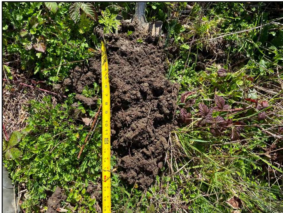
**Photo 8.** View of the soil profile at TP-4 lacking hydric soil indicators.
