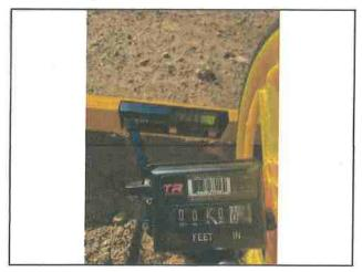
Photo # 857 Prvate Access Rd Slope 29.9% Width 10'
