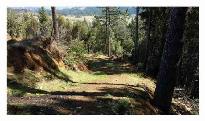
Figure 22. Site number 21, road drainage needed, rolling dip location
