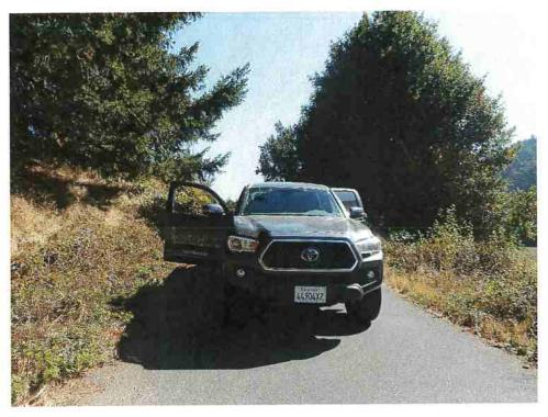
Figure 5: RP4. 14' Paved road width; Inboard ditch and location of lead-out ditch (Left in Image). Image shown facing East.
