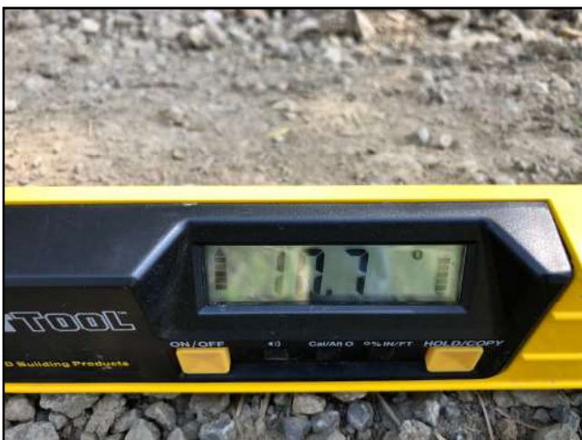
Photo #29 APN 210-074-008 Private Drive Slope 10.7%
