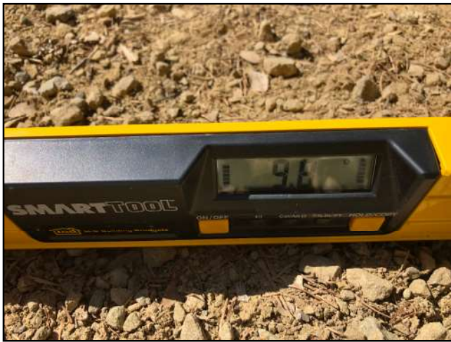
Photo #49 APN 210-074-008 Private Access Rd Slope 9.6%
