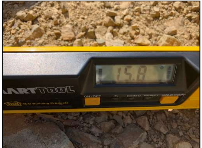
Photo #16 APN 210-074-008 Private Drive Slope 15.8%
