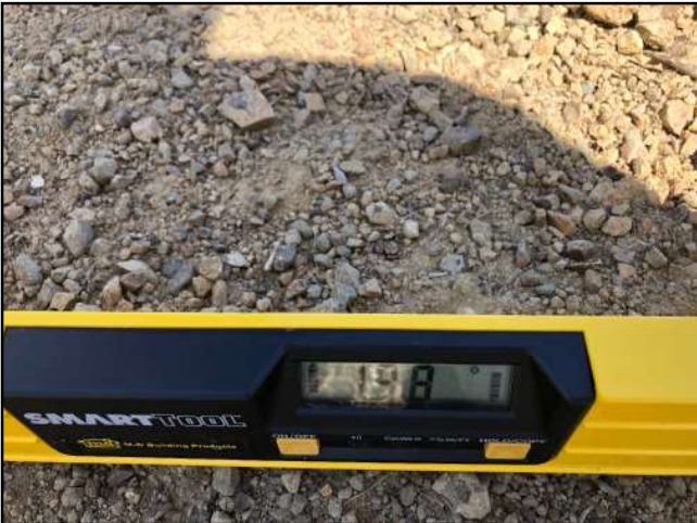
Photo #21 APN 210-074-008 Private Drive Slope 19.8%
