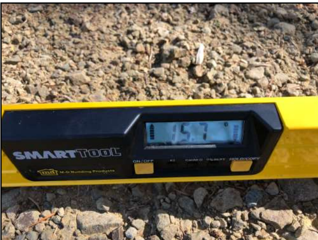
Photo #9 APN 210-074-008 Private Drive Slope 15.7%
