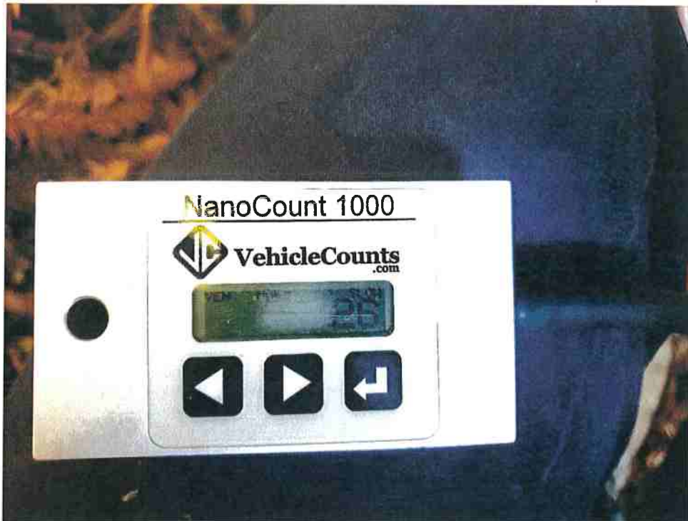
Figure 31: Nanocount 1000 used for 24-hour road study on Warren Creek Road at \langle 124^{\circ}1'30.689''W , 40^{\circ}53'37.41''N \rangle from 11/20/2019 to 11/21/2019, showing final reading of 26 vehicles
