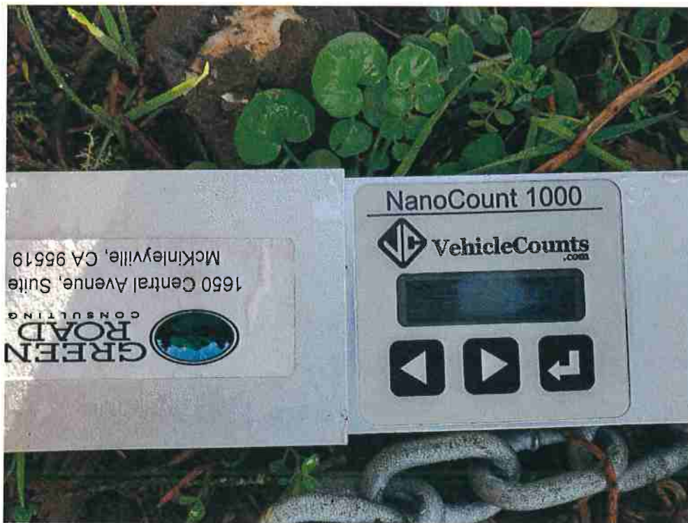
Figure 32: Nanocount 1000 used for 24-hour road study on Warren Creek Road at \langle 124^{\circ}1'54.695''W , 40^{\circ}53'56.232''N \rangle from 1/2/2020 to 1/3/2020, showing final reading of 216 vehicles
