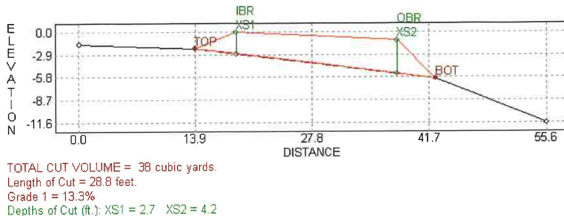
Figure 7. Existing Stream Crossing Fill Prism
