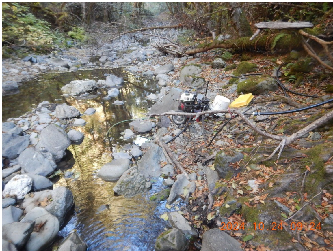
Figure 6. Point 2 – surface water diversion with gas pump in Little Larabee Creek.
