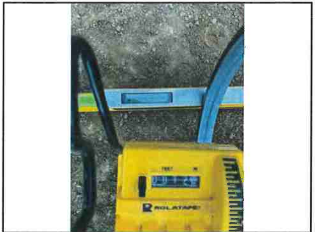
Photo #22 APN #223-034-005 Private Access Rd Width 12'5" Slope 13.2%
