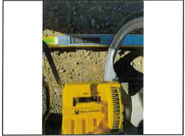
Photo #230 Blue Rock Rd Width 16'3" Slope 9.6%
