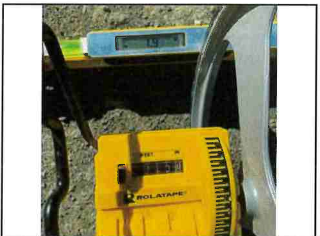
Photo #282 Blue Rock Rd Width 15' 1" Slope 1.9%
