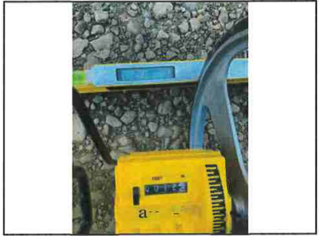
Photo #70 APN #223-034-005 Private Access Rd Width 12'8" Slope 21.7%
