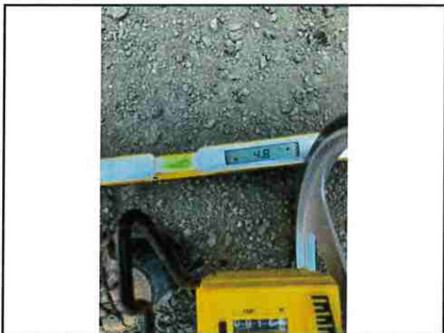
Photo #185 Blue Rock Rd Width 12'3" Slope 4.8%
