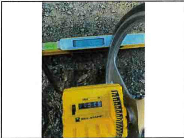
Photo #51 APN #223-034-005 Private Access Rd Width 12'2" Slope 20.4%
