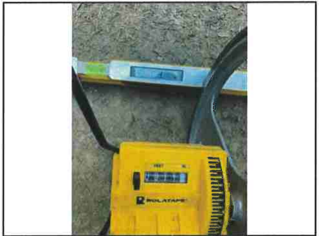
Photo #12 APN #223-034-005 Private Access Rd Width 11'11" Slope 0.3%
