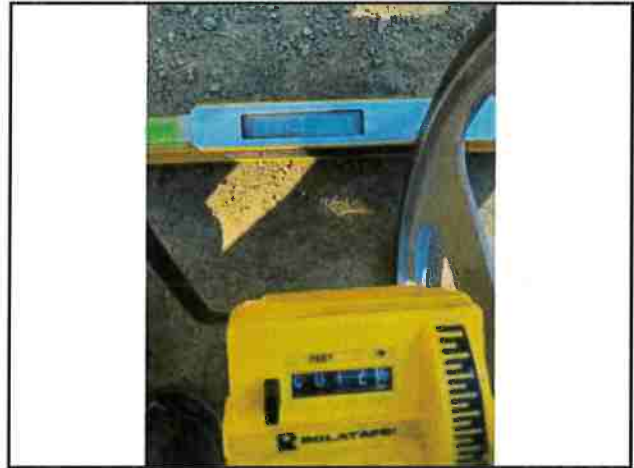
Photo #64 APN #223-034-005 Private Access Rd Width 12'8" Slope 18.8%
