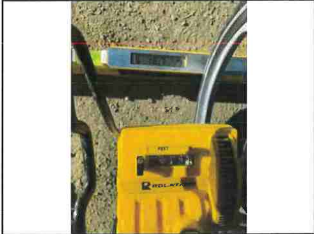
Photo #31 APN #223-034-005 Private Access Rd Width 14'6" Slope 16.7%
