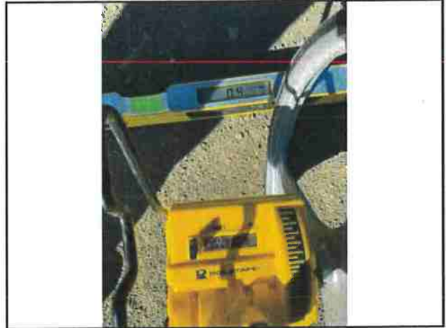
Photo #212 Blue Rock Rd Width 17'1" Slope 0.9%
