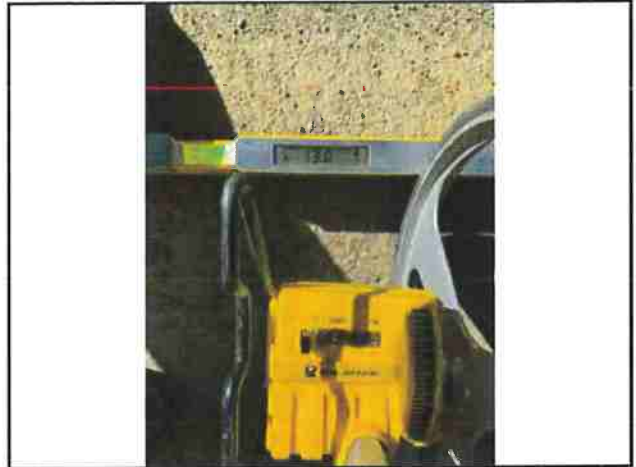
Photo #260 Blue Rock Rd Width 17'3" Slope 13.0%
