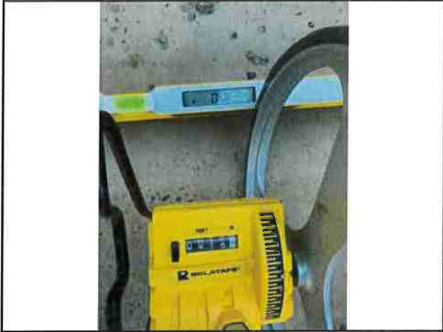
Photo #85 Blue Rock Rd Width 13'0" Slope 0.2%
