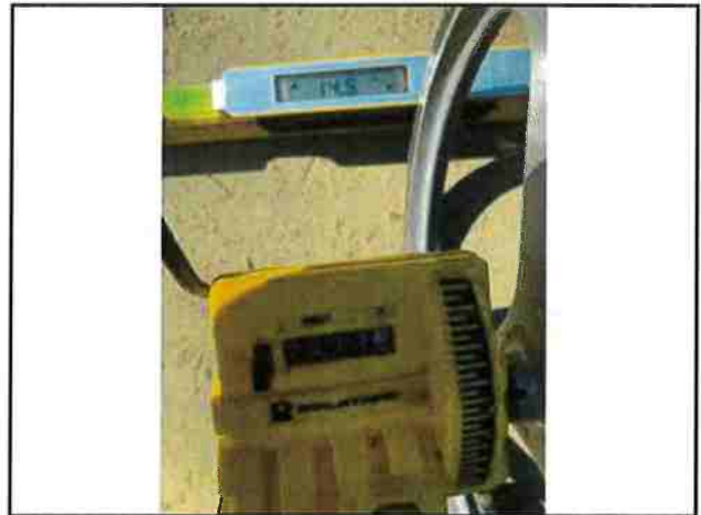
Photo #124 Blue Rock Rd Width 15'6" Slope 14.5%
