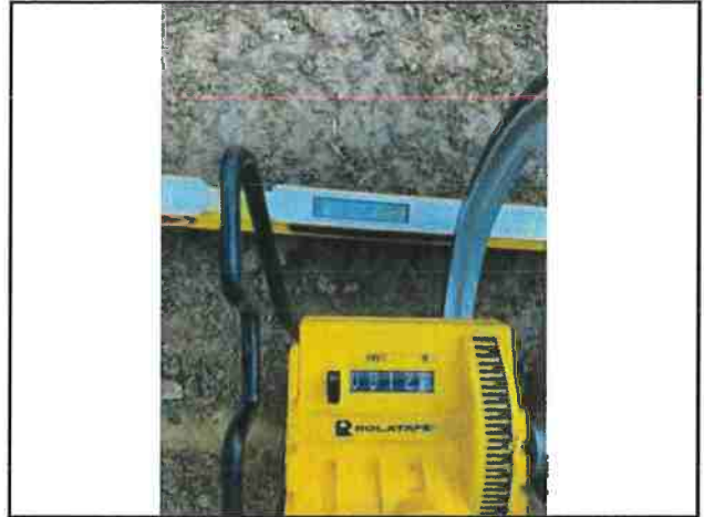
Photo #20 APN #223-034-005 Private Access Rd Width 12'4" Slope 34.2%
