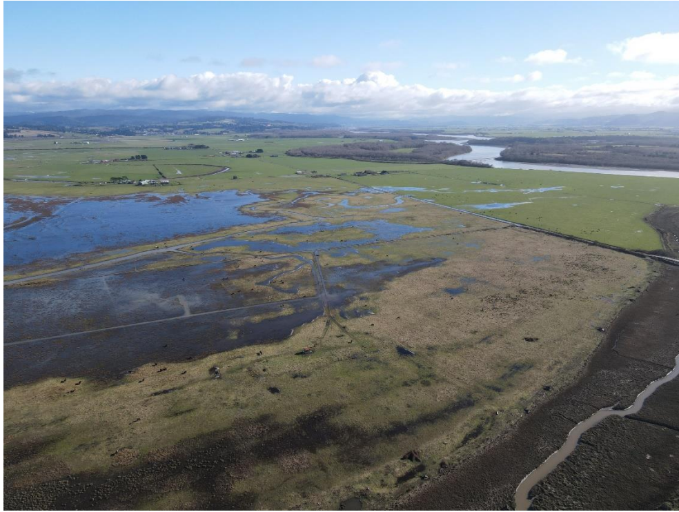
Photo 1—Drone footage from December 2021, looking southeast at Cannibal Island Road. Note flooding in road prism where the elevation has become lower relative to the edges of the pasture to the north and south of the road. Cannibal Island Road is proposed to be elevated in this area during Project implementation.
