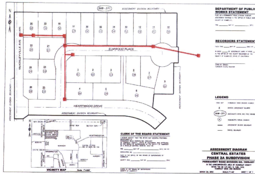
Above: Diagram showing the storm drain system to be maintained by the County as part of the proposed division for road maintenance.
