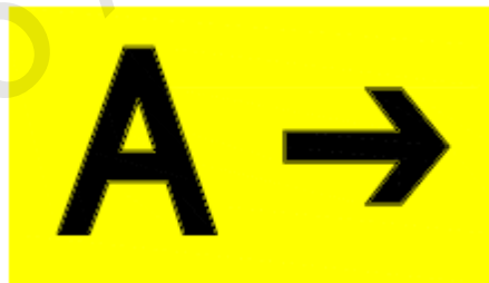
Direction/Runway Exit Sign
