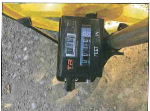
Photo #72 River Rd Width 16.2' @ Turnout
