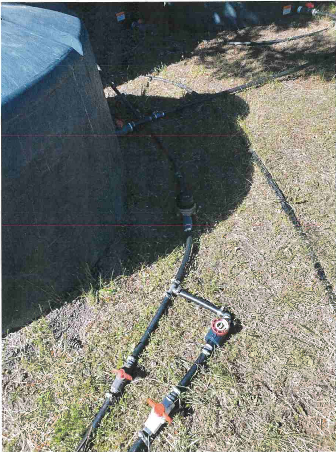
Photo 20. Water gage monitoring diversion from spring. Photo taken Sept 2020.
