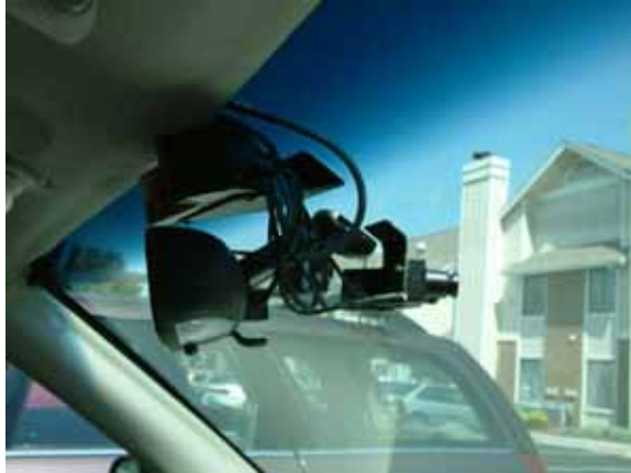
Figure 9. Forward Facing Cameras Mounted Behind the Center Rear View Mirror.
