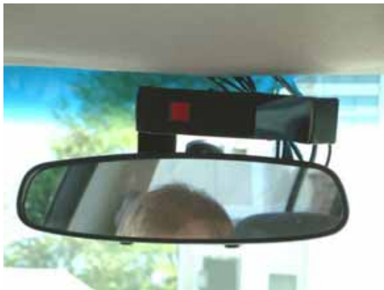
Figure 11. Driver Face Camera Mounted Above Rear View Mirror.
