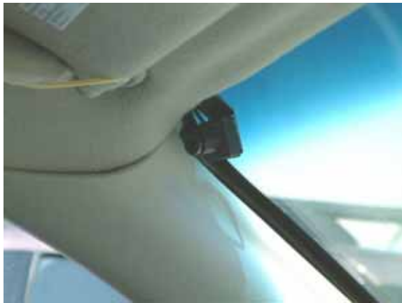
Figure 10. Driver Face Camera, Mounted on the Top Left Corner of the Windshield near the A-Pillar.
