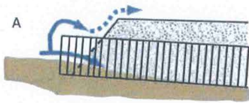
FIGURE 155. Proper culvert installation involves correct culvert orientation, setting the pipe slightly below the bed of the original stream, and backfilling and compacting the fill as it is placed over the culvert. Installing the inlet too low in the stream (A) can lead to culvert plugging, yet if set too high (B) flow can undercut the inlet. If the culvert is placed too high in the fill (C), flow at the outfall will erode the fill. Placed correctly (D), the culvert is set slightly below the original stream grade and protected with armor at the inlet and outlet. Culverts installed in fish-bearing stream channels must be inset into the streambed sufficiently (>25% embedded) to have a natural gravel bottom throughout the culvert (Modified from: MDSL, 1991).
