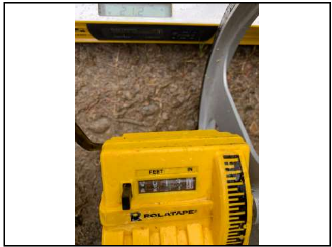
Photo #8 Private Access Rd APN 216-202-009 Width 10'11" Slope 21.2%
