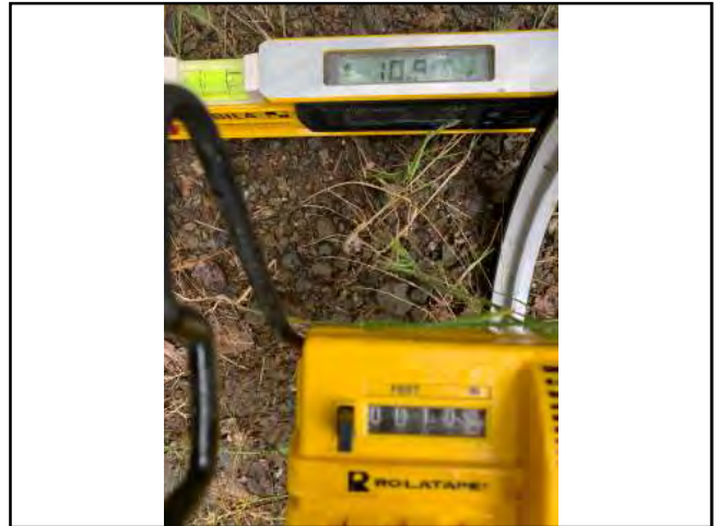
Photo #58 Private Access Rd Width 10'6" Slope 10.9%
