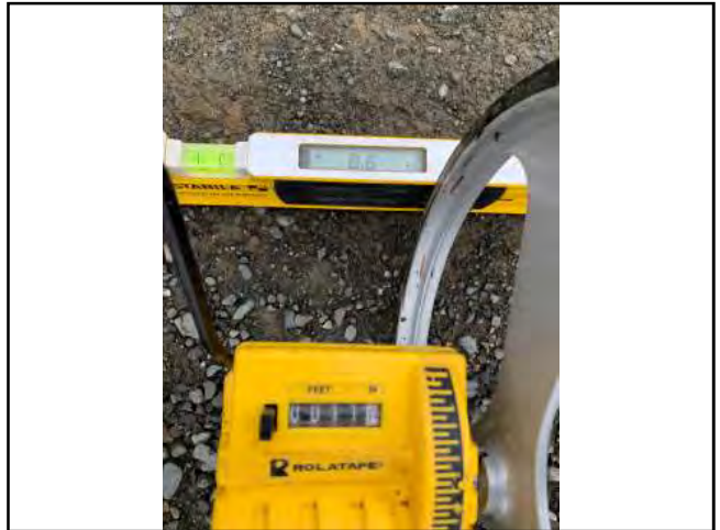
Photo #202 Stewart Ranch Rd Width 11'0” Slope 8.6%
