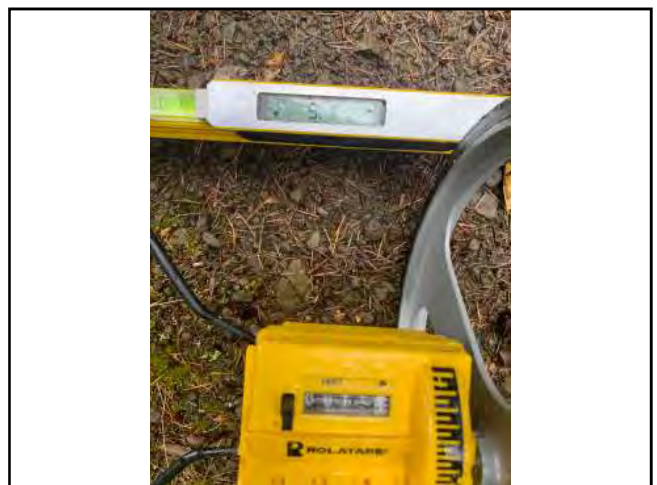
Photo #36 Private Access Rd Width 10'9" Slope 8.2%
