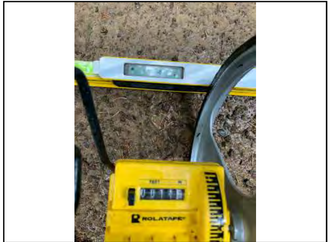
Photo #154 Private Access Rd Width 11'8" Slope 5.4%
