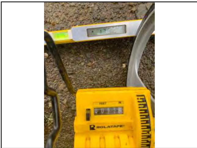
Photo #39 Private Access Rd Width 11'11" Slope 17.5%
