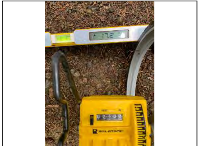
Photo #70 Private Access Rd Width 10'7" Slope 17.2%
