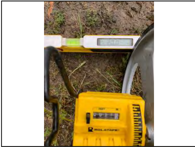
Photo #55 Private Access Rd Width 11'2" Slope 20.0%
