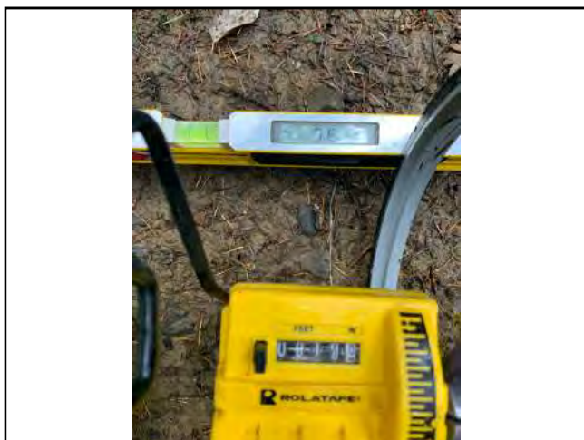
Photo #113 Private Access Rd Width 10'8" Slope 9.6%
