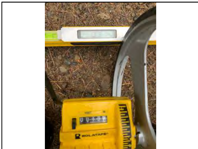
Photo #119 Private Access Rd Width 10'8" Slope 13.3%
