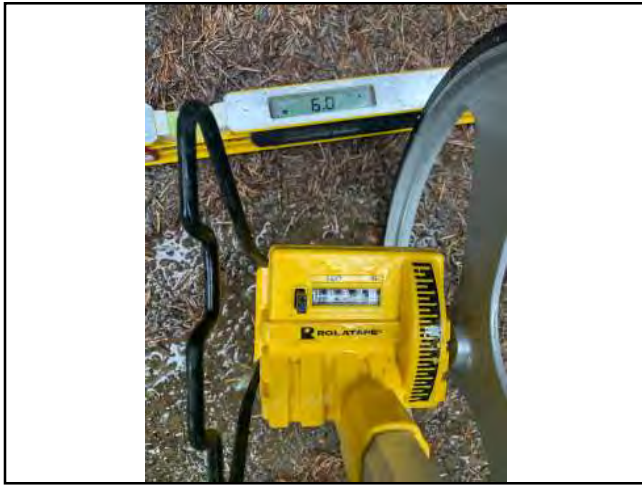
Photo #25 Private Access Rd APN 216-202-009 Width 12'1" Slope 6.0%
