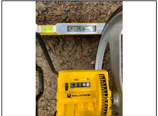
Photo #94 Private Access Rd Width 10'0" Slope 15.8%
