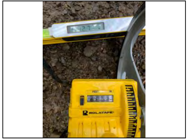
Photo #104 Private Access Rd Width 10'3" Slope 12.7%
