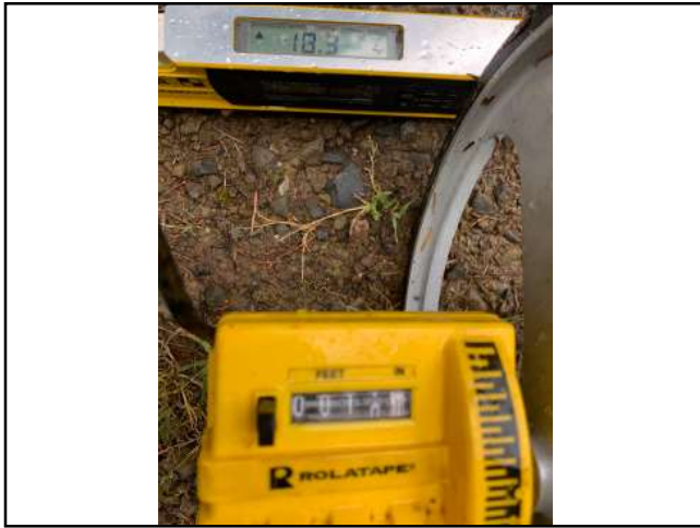
Photo #127 Private Access Rd Width 10'11" Slope 18.3%
