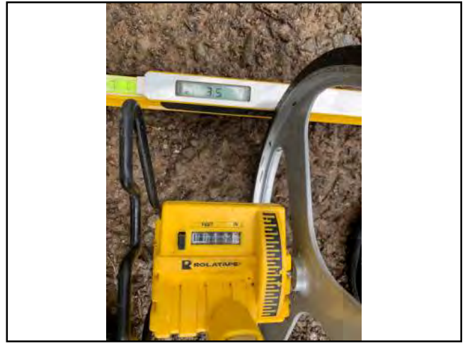
Photo #176 Private Access Rd Width 11'8" Slope 3.5%
