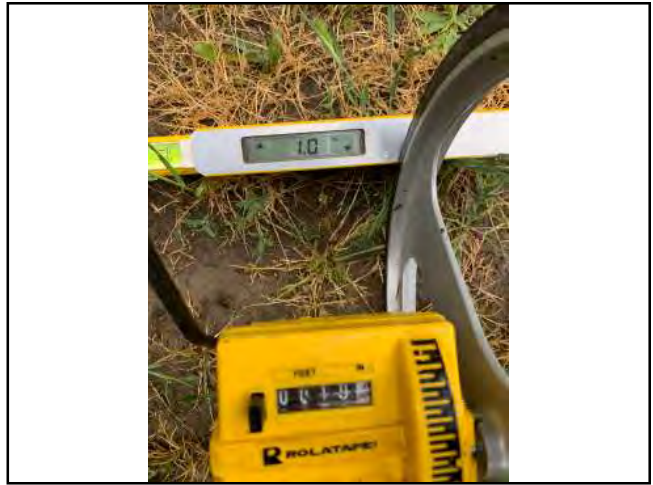
Photo #110 Private Access Rd Width 10'4" Slope 1.0%
