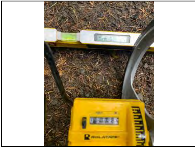
Photo #73 Private Access Rd Width 10'8" Slope 14.8%
