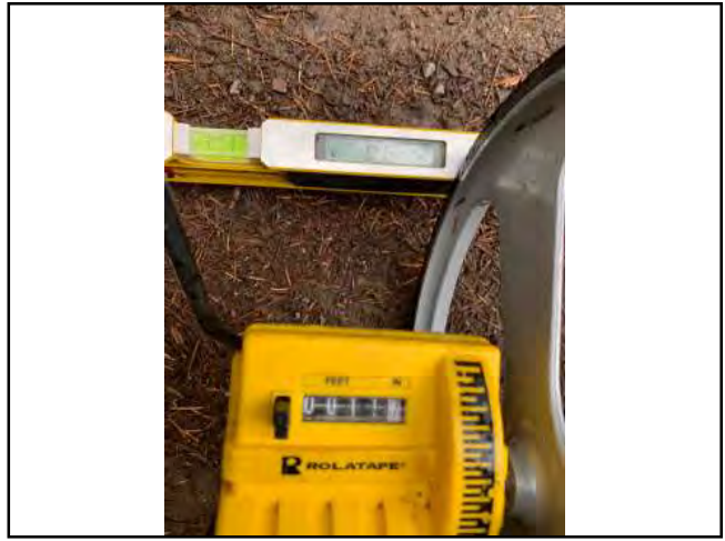
Photo #146 Private Access Rd Width 11'7" Slope 0.6%
