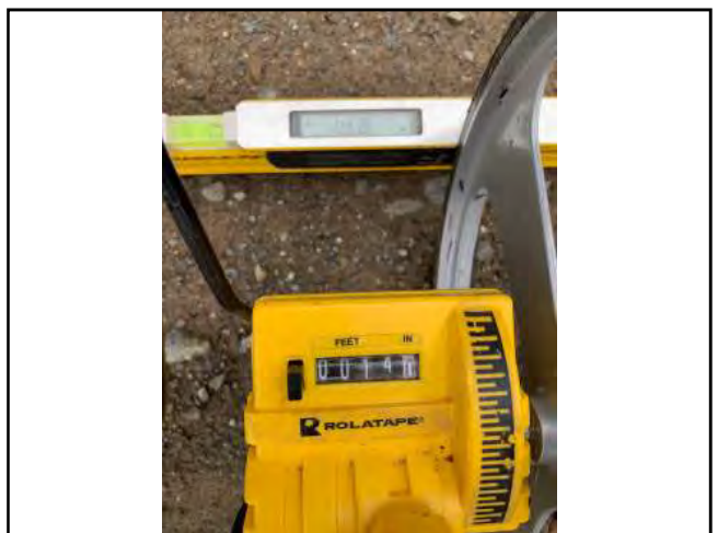
Photo #216 Stewart Ranch Rd Width 14'0" Slope 14.8%
