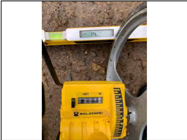
Photo #213 Stewart Ranch Rd Width 14'4" Slope 14.2%
