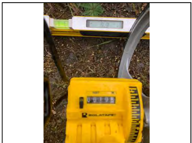
Photo #42 Private Access Rd Width 10'3" Slope 9.3%
