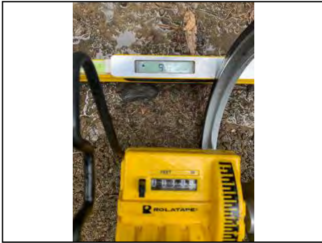
Photo #61 Private Access Rd Width 10'6" Slope 10.9%
