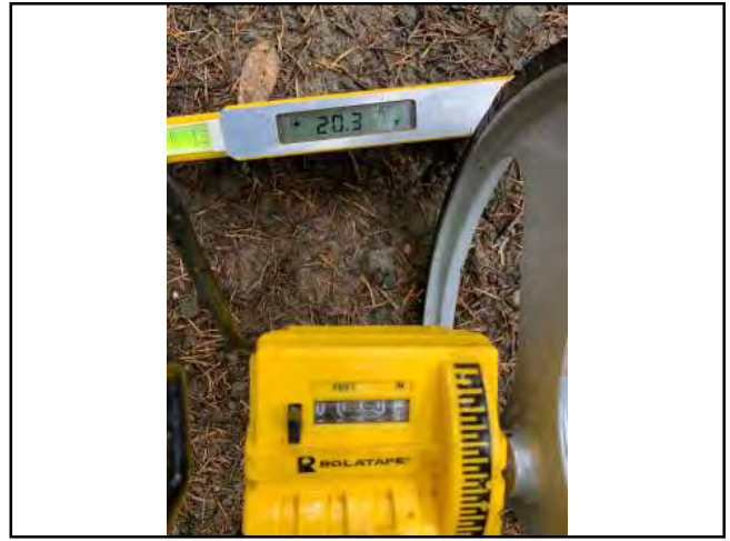
Photo #80 Private Access Rd Width 10'2" Slope 20.3%
