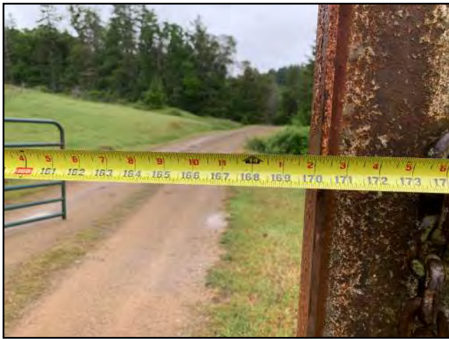
Photo #163 Private Access Rd Gate Width 14'2"
