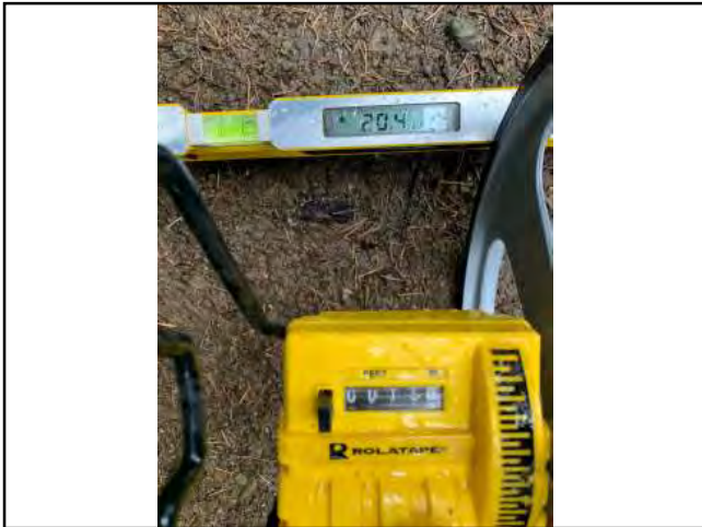
Photo #15 Private Access Rd APN 216-202-009 Width 11'0" Slope 20.4%
