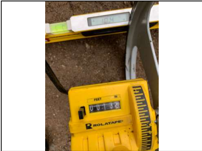
Photo #207 Stewart Ranch Rd Width 13'5" Slope 10.4%
