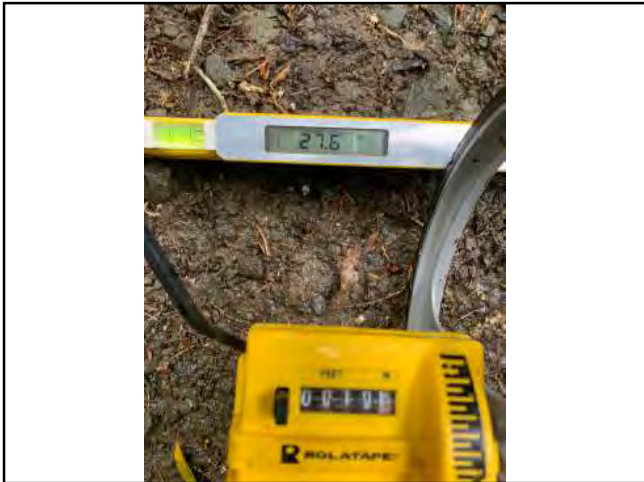
Photo #99 Private Access Rd Width 10'2" Slope 27.6%
