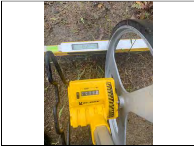
Photo #31 Private Access Rd Width 10'9" Slope 8.2%
