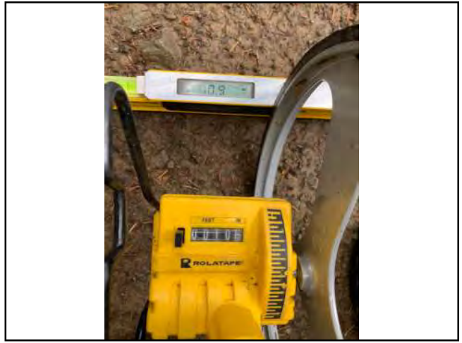
Photo #188 Private Access Rd Width 10'8" Slope 10.9%
