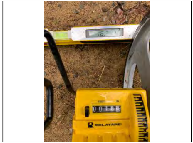
Photo #122 Private Access Rd Width 10'8" Slope 16.3%
