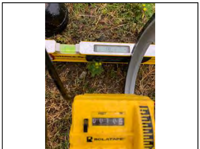
Photo #6 Private Access Rd APN 216-202-009 Width 10'2" Slope 19.1%
