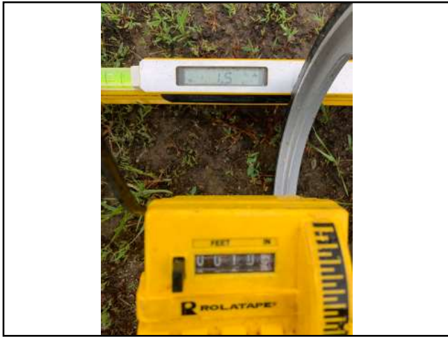
Photo #49 Private Access Rd Width 10'3" Slope 9.3%
