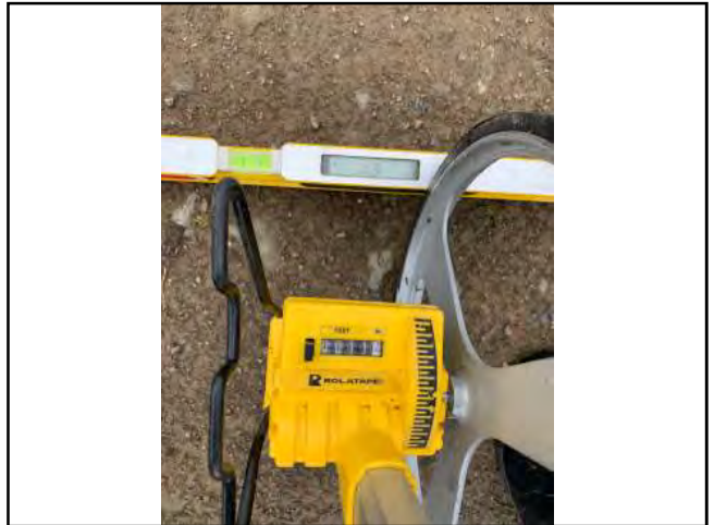
Photo #196 Private Access Rd Width 11'4” Slope 1.3%
