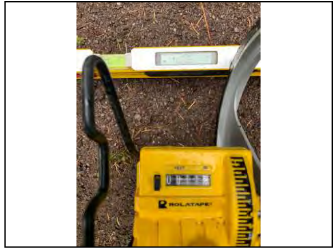
Photo #140 Private Access Rd Width 11'1" Slope 17.6%
