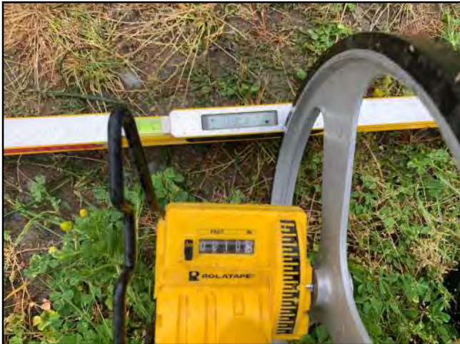
Photo #3 Private Access Rd APN 216-202-009 Width 10'4" Slope 13.1%
