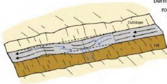
Type 1 rolling dips are used where road grades are less than about 12-14% and road runoff is not confined by a large through cut or berm. The axis of the dip should be perpendicular to the road alignment and sloped at 3-4% across the road tread. Steep roads will have longer and more abrupt dip dimensions to develop reverse grade through the dip axis. The road tread and/or the dip outlet can be rocked to protect against erosion, if needed.
