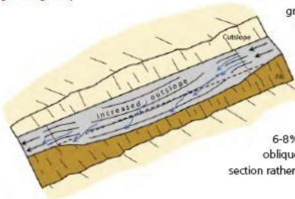
Type 3 rolling dips are utilized where road grades are steeper than about 12% and it is not feasible to develop a reverse grade that will also allow passage of the design vehicle (steep road grades require more abrupt grade reversals that some vehicles may not be able to traverse without bottoming out).
