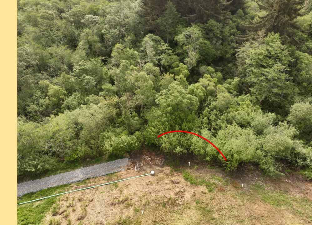
Photo was taken on November 12<sup>th</sup>, 2025, showing the current state of the southern access road. Only limited willow removal was necessary adjacent to the road to give enough clearing for the extension of the Southern Access Road. Several willows were removed towards the end of the Southern Access Road, and the vegetation line was retreated, to keep the woody roots off of the landfill cap and away from the subterranean leachate collection system.
