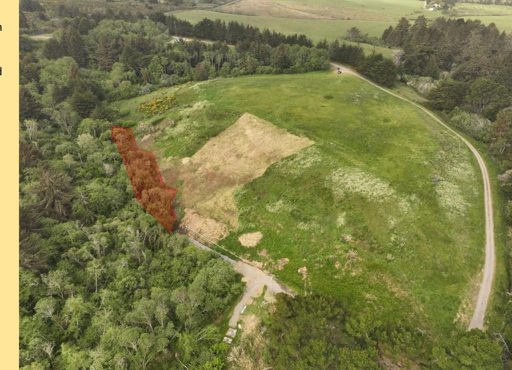
Another aerial drone imagery, showing the encroachment of the willows onto the landfill cap. This area will be addressed by retreating/removing the willows off of the cap in 2026. Encroaching willows shown in red.
