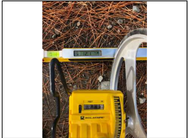
Photo #166 Private Access Rd Slope 12.1% Width 10'5"
