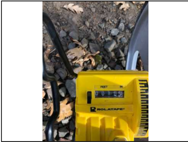
Photo #151 Private Access Rd @ Intersection of other Private Road Width 10'6"
