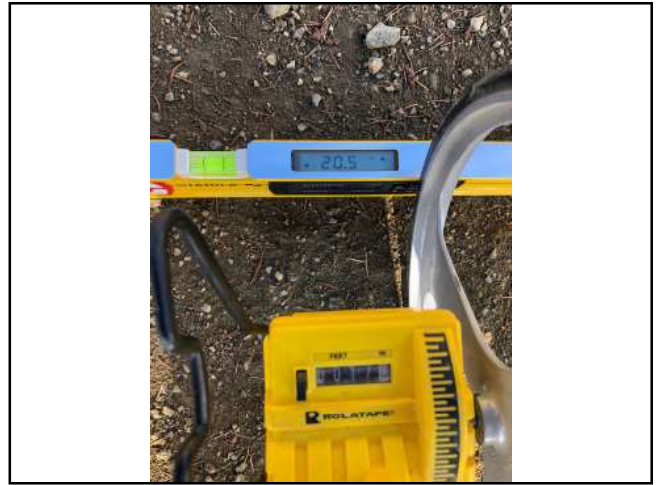
Photo #211 Private Access Rd S;lope 20.5% Width @ Pullout 17'0"
