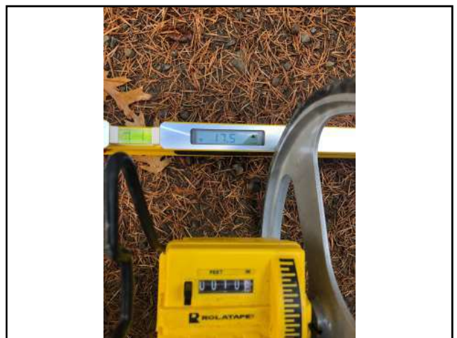
Photo #138 Private Drive Slope 17.5% Width 10'3"
