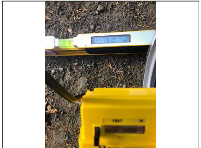
Photo #118 Private Access Rd Slope 19.0% Width 11'1"
