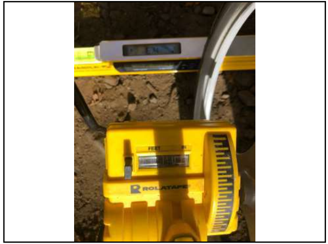
Photo #104 Driveway Slope 6.4% Width 10'6"
