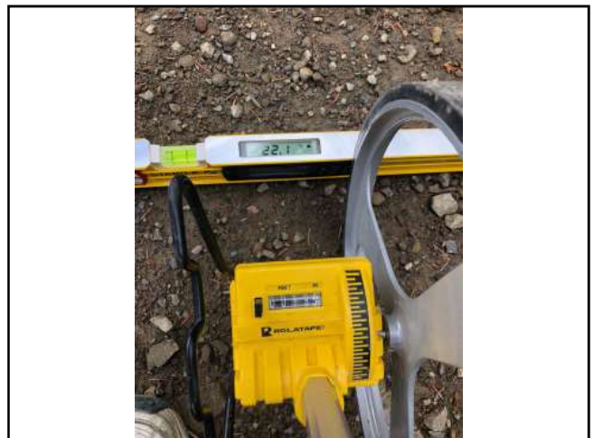
Photo #257 Private Access Rd Slope 22.1% Width 19'6" @ Pullout
