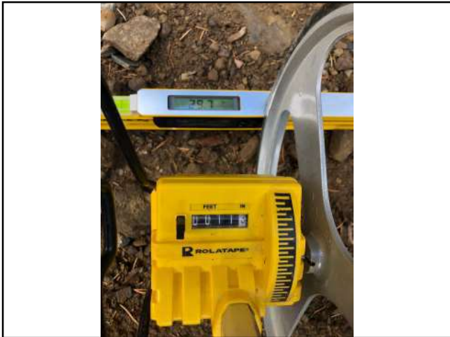
Photo #248 Private Access Rd slope 29.7% Width 11'3"
