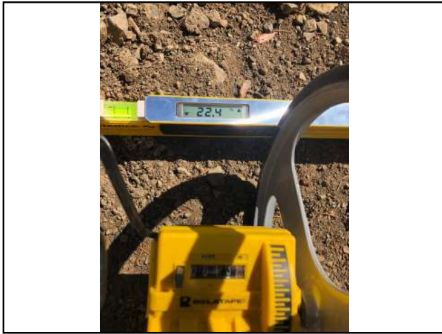
Photo #228 Private Access Rd Slope 22.4% Width 13'0"
