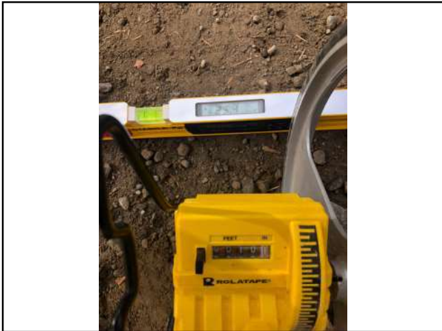
Photo #93 Private Access Rd Slope 25.4% Width 10'0"
