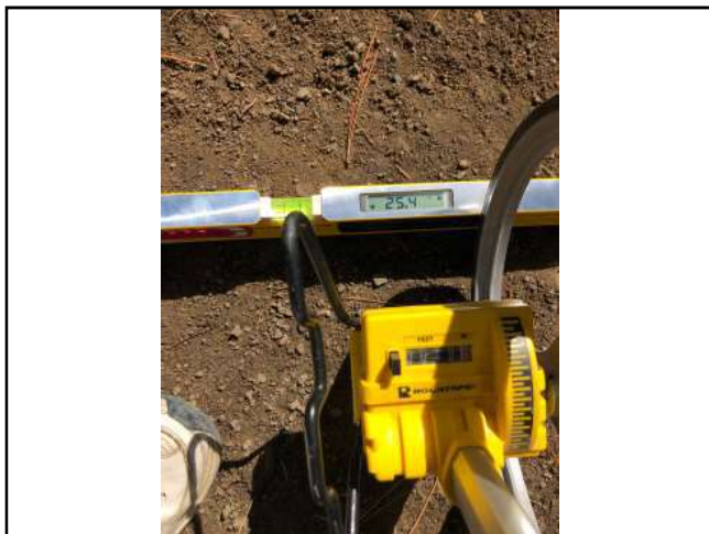
Photo #238 Private Access Rd Slope 25.4% Width 10'10"
