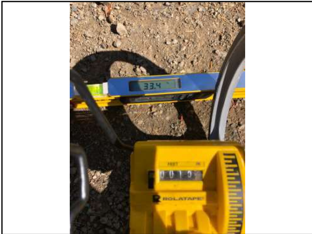
Photo #224 Private Access Rd Slope 33.4% Width 15'5"
