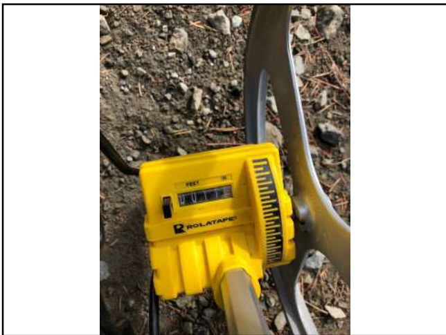
Photo #171 Private Access Rd Width After Pullout 11'9"
