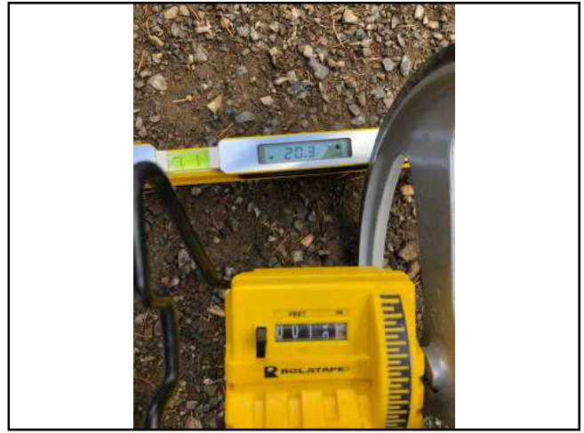
Photo #253 Private Access Rd Slope 20.3% Width 12'11"
