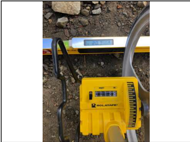
Photo #242 Private Access Rd Slope 20.3% Width 18'4" @ Pullout
