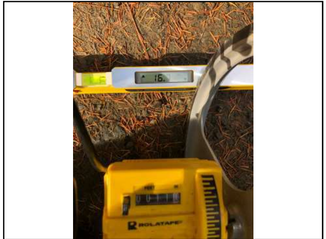
Photo #142 Private Drive Slope 16.7% Width 11'10"
