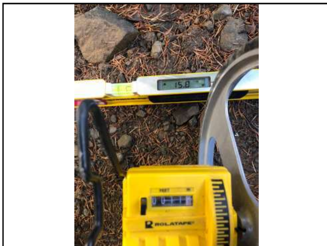
Photo #131 Private Access Rd Slope 15.8% Width 11'1"
