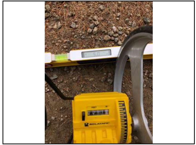
Photo #277 Private Access Rd Slope 5.0% Width 11'0"
