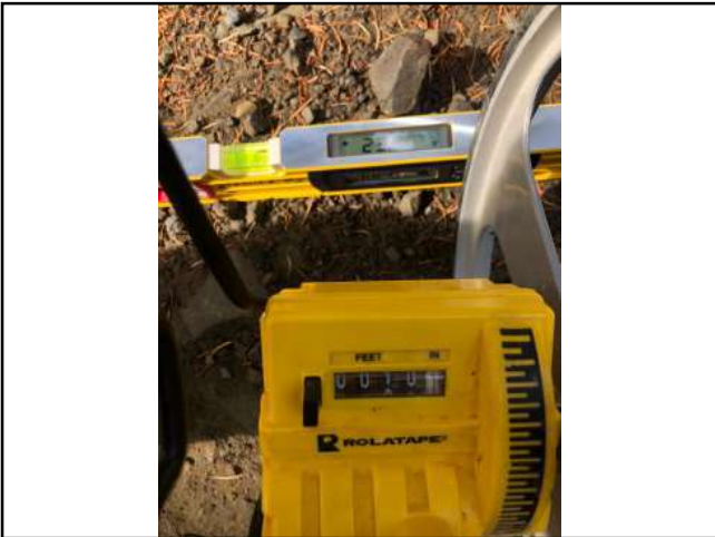
Photo #81 Private Access Rd slope 23.4% Width 10'1"
