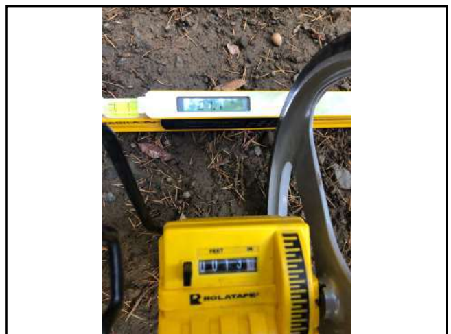
Photo #245 Private Access Rd Slope 27.1% Width 13'1"
