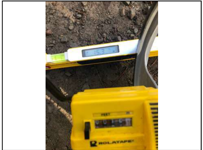
Photo #106 Private Access Rd Slope 5.3% Width 12'1"
