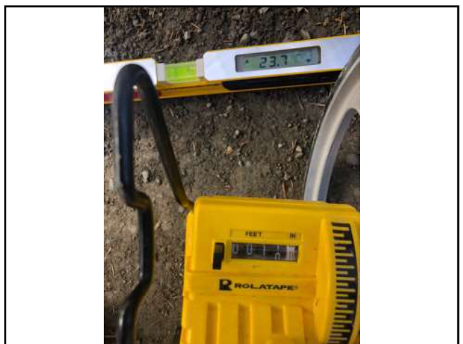
Photo #126 Private Access Rd Slope 23.7% Width 10'1"
