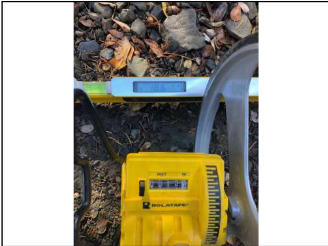
Photo #230 Private Access Rd Slope 18.6% Width 15'4"
