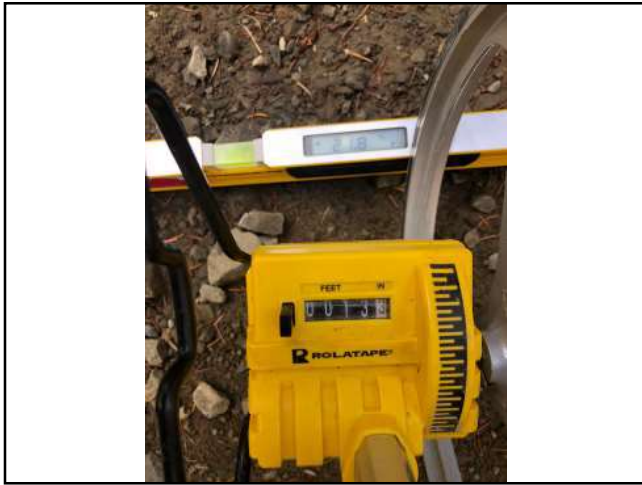
Photo #181 Private Access Rd Slope 21.8% Width 13'3"
