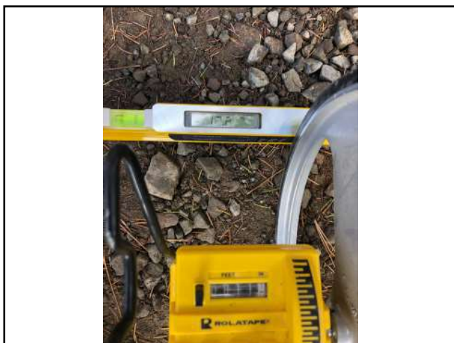
Photo #173 Private Access Rd Slope 12.8% Width 11'1"
