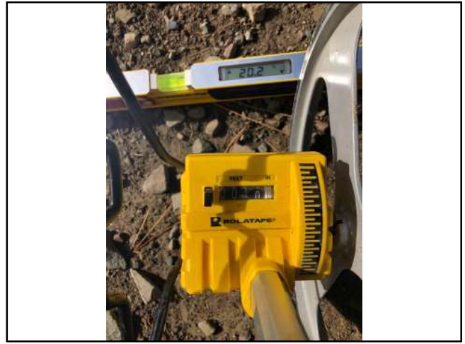
Photo #176 Private Access Rd Slope 20.2% Width 10'11"
