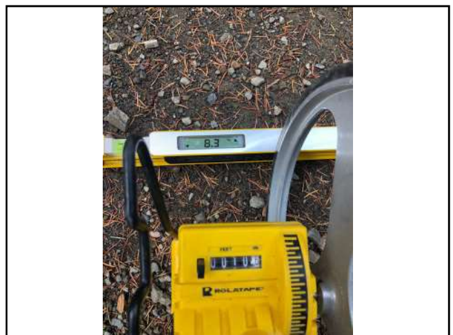
Photo #263 Private Access Rd Slope 8.3% Width 10'6"
