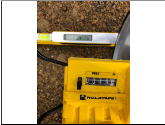
Photo #19 Private Driveway On APN 216-381-021 Slope 11.4% Width 14'5"
