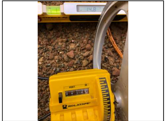
Photo #10 River Dr Slope 14.8% Width 13'5"
