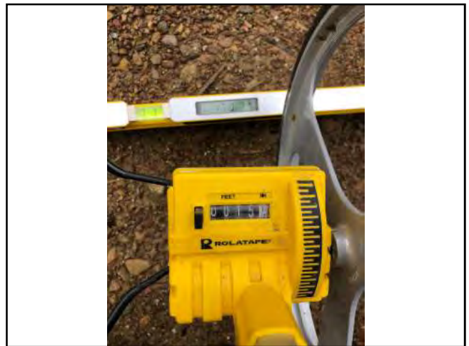
Photo #16 Private Driveway On APN 216-381-021 Slope 17.0% Width 15'11"
