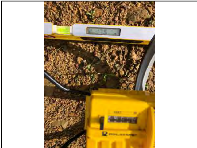
Photo #21 Private Driveway On APN 216-381-021 Slope 17.5% Width 14'1"
