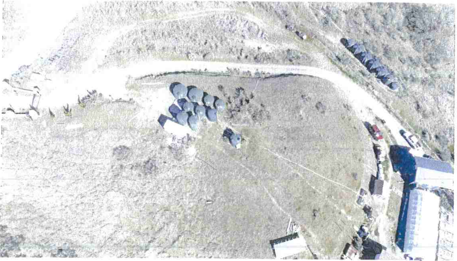
Picture 7: Tank Farm south of driveway consisting of four 5,000 gallon plastic tanks, four 3,000 gallon plastic tanks, and two 2,850 gallon plastic tank. Total storage at this site is 37,700 gallons. Tank Farm north of driveway consisting of four 2,850 gallon plastic tanks, two 3,000 gallon plastic tanks, and one 1,550 gallon plastic tank. Total storage at this site is 21,800 gallons. Photo date 2-17-2018.
