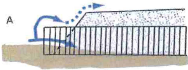
FIGURE 155. Proper culvert installation involves correct culvert orientation, setting the pipe slightly below the bed of the original stream, and backfilling and compacting the fill as it is placed over the culvert. Installing the inlet too low in the stream (A) can lead to culvert plugging, yet if set too high (B) flow can undercut the inlet. If the culvert is placed too high in the fill (C), flow at the outfall will erode the fill. Placed correctly (D), the culvert is set slightly below the original stream grade and protected with armor at the inlet and outlet. Culverts installed in fish-bearing stream channels must be inset into the streambed sufficiently (>25% embedded) to have a natural gravel bottom throughout the culvert (Modified from: MDSL, 1991).
