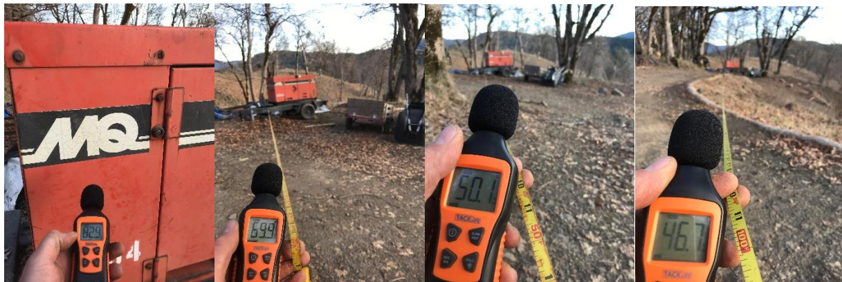
MQ 15 kW generator noise measurements (dB's) at 0 ft, 25 ft, 50 ft, and 100 ft.
