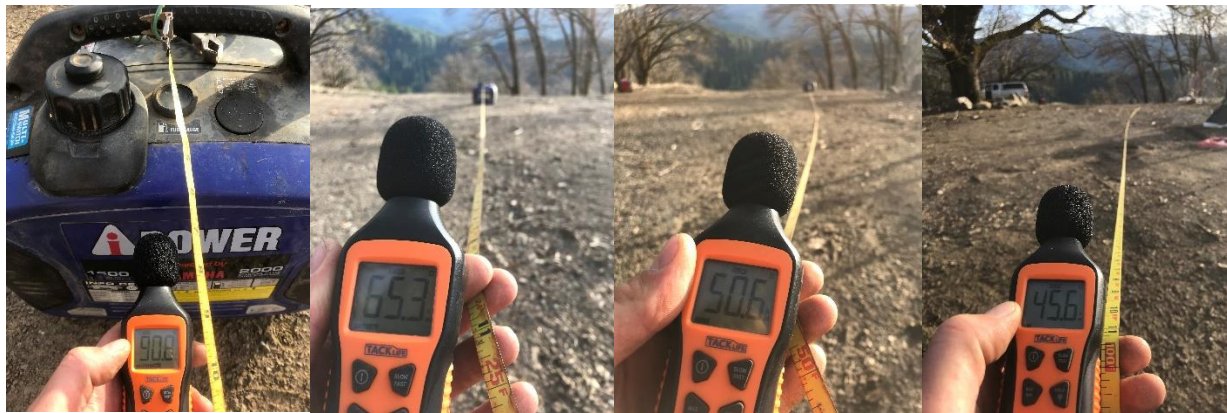
Yamaha iPower generator noise measurements (dB's) at 0 ft, 25 ft, 50 ft, and 100 ft.
