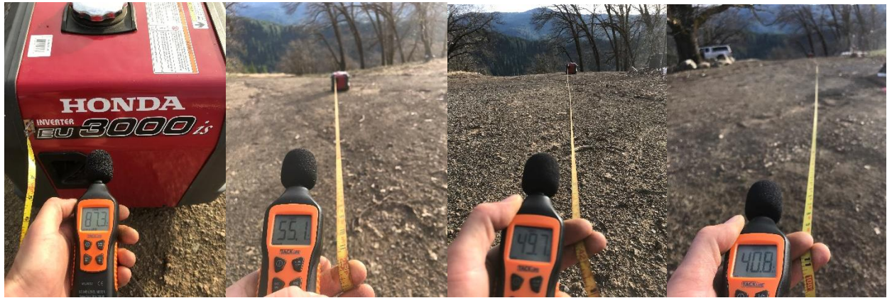
Honda EU 3000i generator noise measurements (dB's) at 0 ft, 25 ft, 42 ft, and 100 ft.
