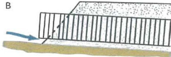
FIGURE 155. Proper culvert installation involves correct culvert orientation, setting the pipe slightly below the bed of the original stream, and backfilling and compacting the fill as it is placed over the culvert. Installing the inlet too low in the stream (A) can lead to culvert plugging, yet if set too high (B) flow can undercut the inlet. If the culvert is placed too high in the fill (C), flow at the outfall will erode the fill. Placed correctly (D), the culvert is set slightly below the original stream grade and protected with armor at the inlet and outlet. Culverts installed in fish-bearing stream channels must be inset into the streambed sufficiently (>25% embedded) to have a natural gravel bottom throughout the culvert (Modified from: MDSL, 1991).
