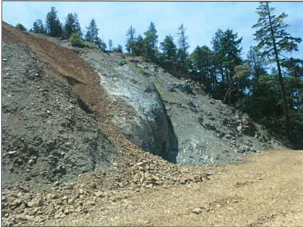
Upper mafic block showing gradation from serpentinite to diabase (left to right)
