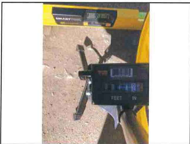
Photo #113 River Rd Slope 9.1% Width 14.6'
