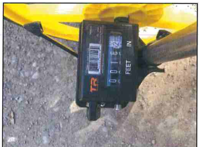
Photo #72 River Rd Width 16.2' @ Turnout
