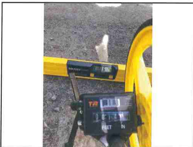
Photo #131 River Rd Slope 3.6% Width 14.1'
