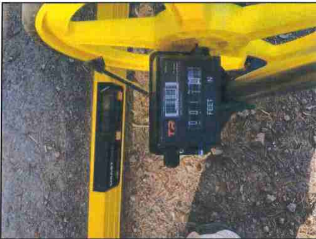
Photo #399 River Rd Slope 10.9% Width 12.0'
