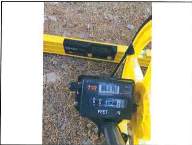
Photo #441 River Rd Slope 16.1% Width 12.4'
