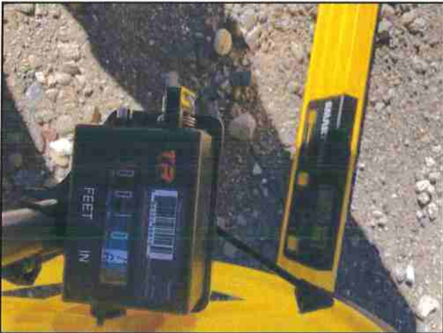
Photo #81 River Rd Slope 9.0% Width 10.7'
