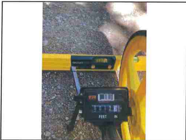
Photo #183 River Rd Slope 11.0% Width 12.7'
