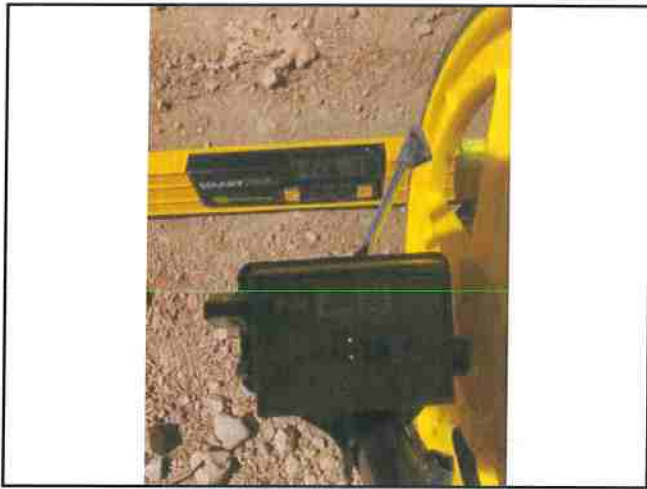
Photo #118 Private Access Rd APN 208-221-014 Slope 22.6% Width 10'11"
