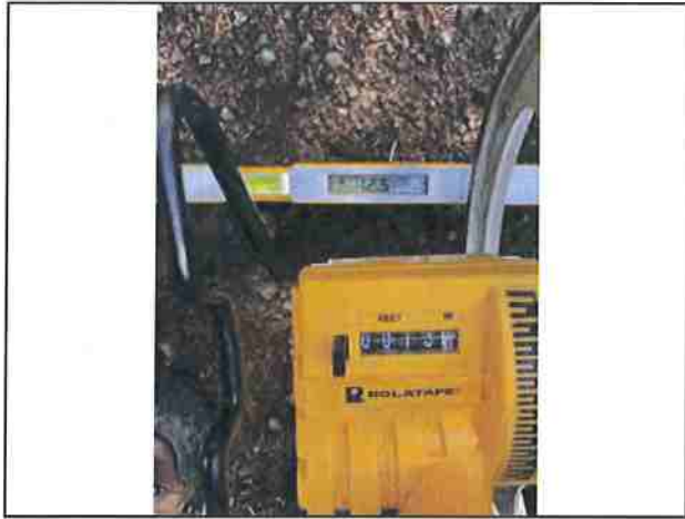
Photo #181 Kings Peak Rd Slope 12.5% Width 13'1"
