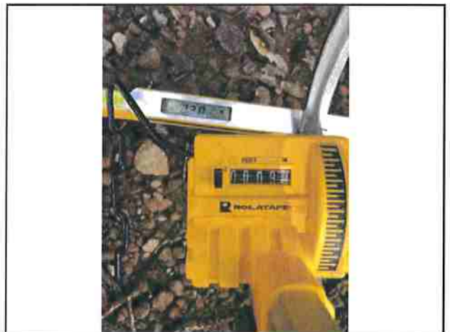
Photo #24 Private Access Rd Width 9'7" Slope 22.0%
