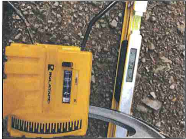
Photo #62 Kings Peak Rd Slope 12.8% Width 14'7"
