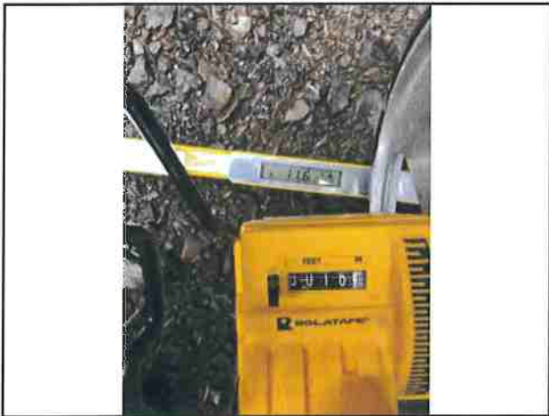
Photo #155 Kings Peak Rd Slope 11.6% Width 16'10"
