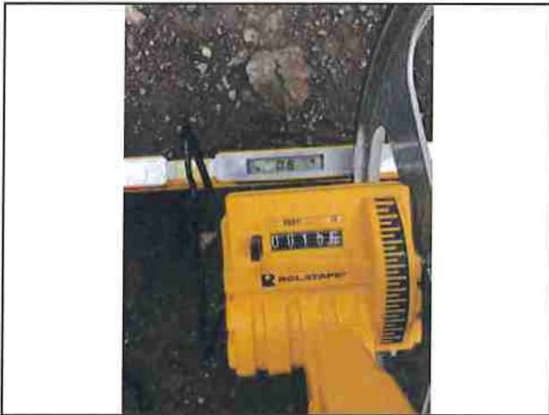
Photo #201 Kings Peak Rd Slope 0.8% Width 15'6"
