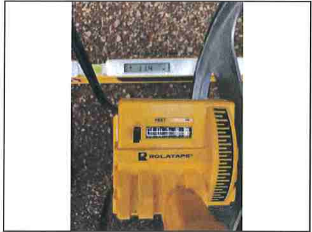
Photo #212 Kings Peak Rd Slope 11.4% Width 16'7"
