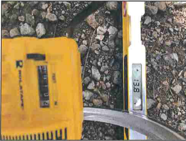
Photo #93 Kings Peak Rd Slope 13.8% Width 18'2"
