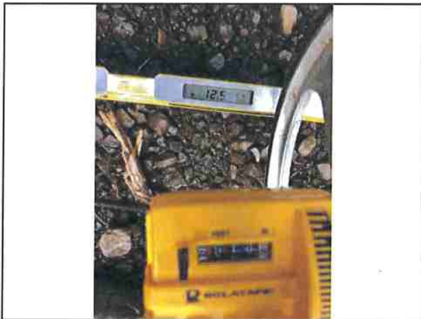
Photo #165 Kings Peak Rd Slope 12.5% Width 18'9"
