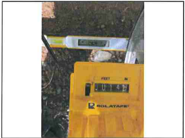
Photo #84 Kings Peak Rd Slope 14.4% Width 14'9"
