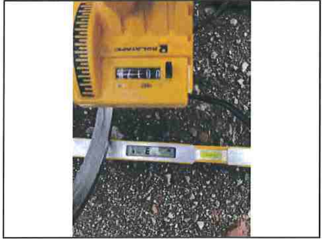
Photo #136 Kings Peak Rd Slope 12.8% Width 17'11"
