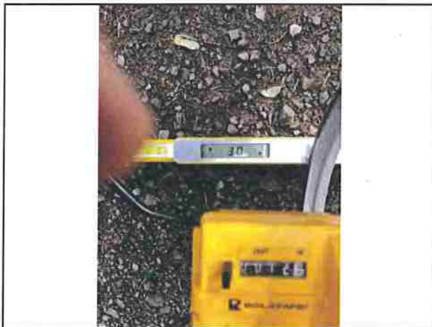
Photo #147 Kings Peak Rd Slope 3.0% Width 12'8"
