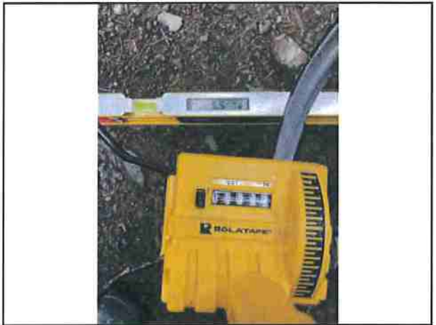
Photo #114 Kings Peak Rd Slope 5.5% Width 11'8"
