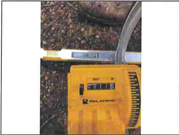
Photo #183 Kings Peak Rd Slope 11.4% Width 17'2"
