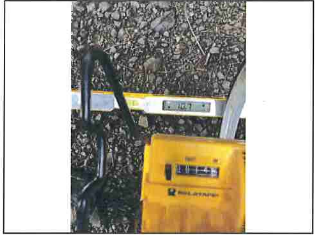
Photo #152 Kings Peak Rd Slope 10.7% Width 14'5"
