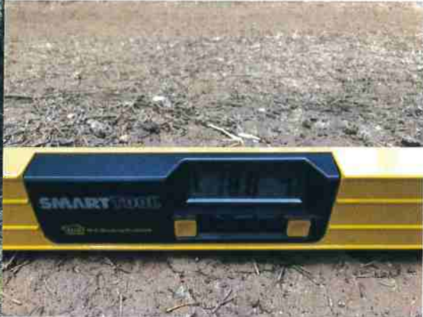
Photo #14 Access Rd Location with Grade Greater Than 16%
