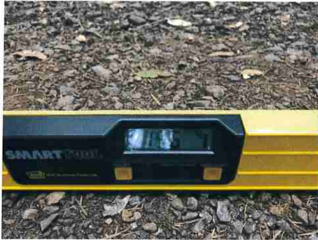
Photo #57 Access Rd @ Grade Steeper Than 16%
