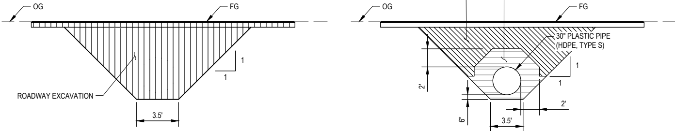
J ROADWAY CROSSING CULVERT EXCAVATION AND BACKFILL NOT TO SCALE
