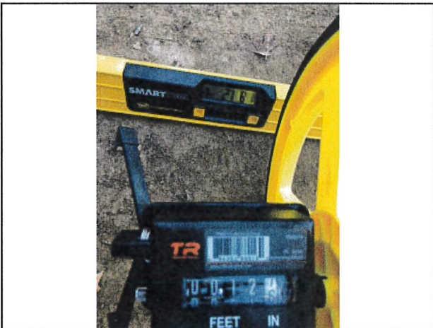
Photo #502 Private Access Rd APN 208-231-012 Slope 21.8% Width 12'6"
