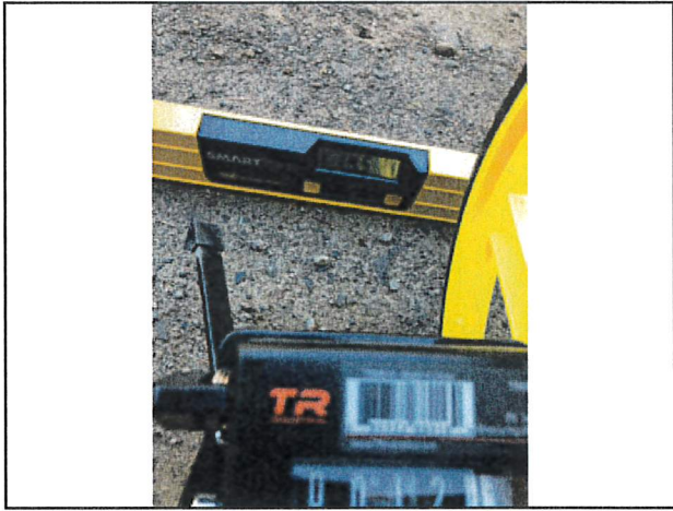
Photo #193 Slope 14.5% Width 12.0' ver Rd
