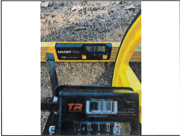
Photo #518 Private Access Rd APN 208-231-012 Slope 18.8% Width 10'2"
