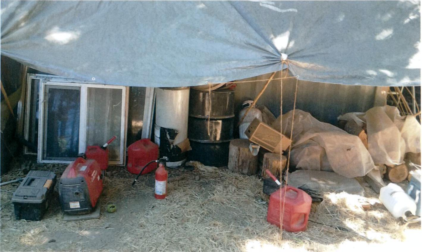
Picture 10: This is a picture of the fuel storage area on the property as of September, 2016. Fuel storage is not in compliance due to lack of secondary containment and protection against wind driven precipitation. The tarped awning will protect against most rain storms, but would not be enough during heavy, wind driven, rain storms. Photo date 9/16/2016
