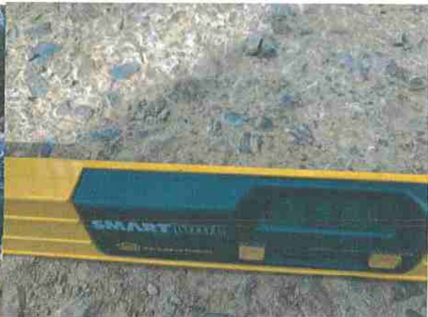
Photo #252, location 64 longitudinal slope = 6.0%.
