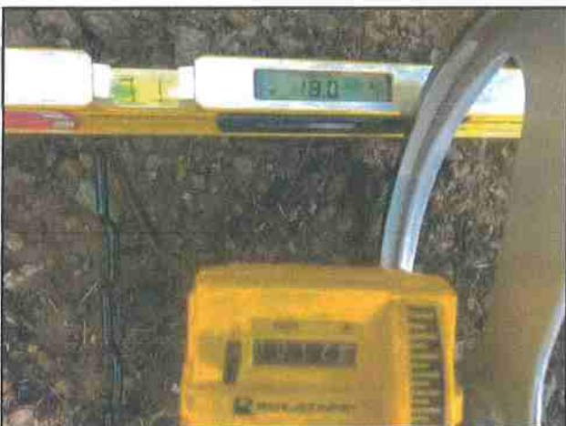
Photo #5 Private Driveway APN 216-382-028 Slope 18.0% Width 12'4"
