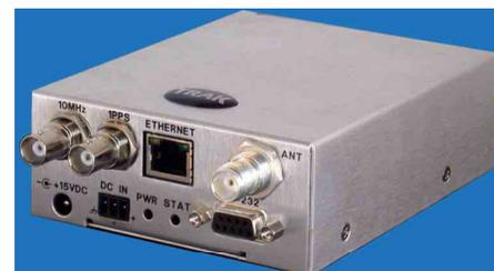
receiver, disciplined oscillator and time and frequency signal generation in a small form factor enclosure.
