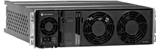
The comparator features a digital or analog voting methodology: Frame Diversity Reception. The comparator selects the data frame or signals with the lowest Bit Error Rate (BER) and forwards it. By using the best pieces of each input signal, the result is the best possible composite signal. This signal is then redistributed across the radio IP network to every connected base station for rebroadcasting.
