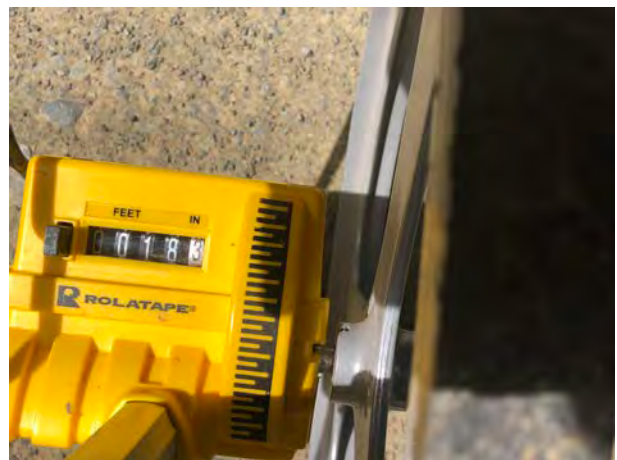
Photo #204 Access Road Width 18'
