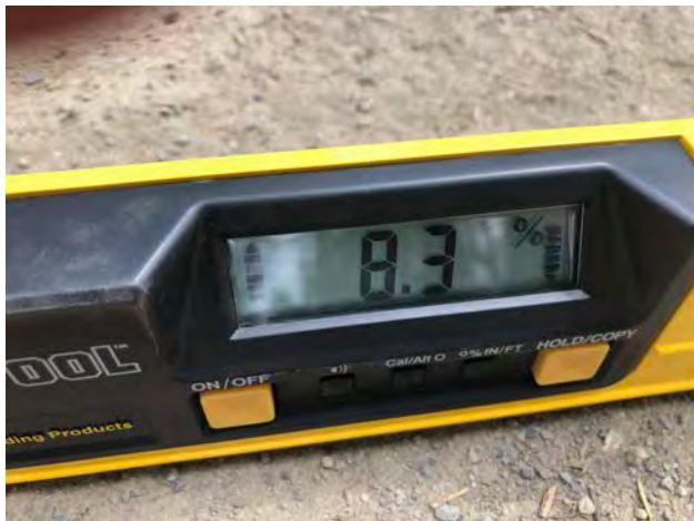
Photo #59 Access Road Slope 8%
